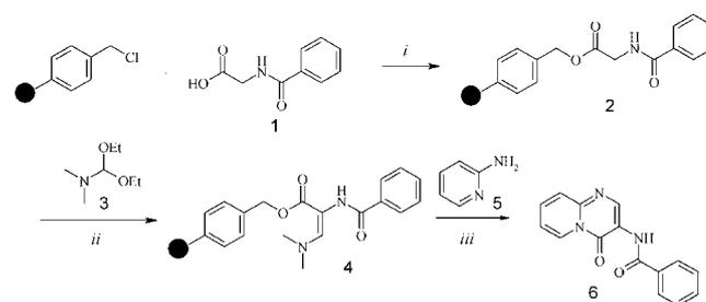
Scheme 3 Synthesis of 3-(benzoyl)amino-4*H*-pyrido[1,2-*a*]pyrimidin-4-one. Reaction conditions: (i) Hippuric acid (5 equiv), CsCO<sub>3</sub> (5 equiv), DMF, 200 °C, 10 min. (ii) DMFDEA (5 equiv) in DMF, 180 °C, 10 min (iii) 2-aminopyridine (0.5 equiv) in HOAc, 180 °C, 10 min.
