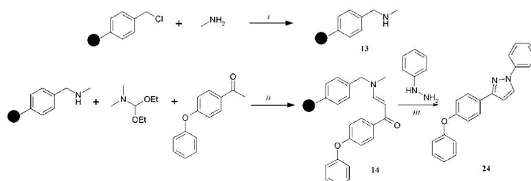
**Scheme 6** Example of a solid phase synthesis of 1-Phenyl-5-(4-phenoxyphenyl)-pyrazole. Reaction conditions: (i) MeNH<sub>2</sub> in H<sub>2</sub>O, 150 °C, 10 min (ii) DMF, 150 °C, 10 min (iii) HOAc, 150 °C, 10 min.
