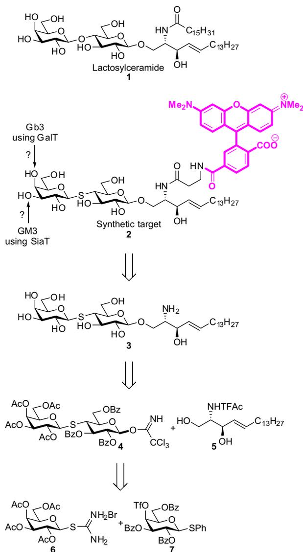
**Scheme 1.** Retrosynthesis of target **2** having a sulfur linkage between galactose and glucose.
