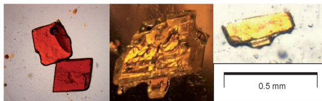
**Figure 1.** Microscope images of single crystals of the complex nitrates  $(\text{NO})_2[\text{Pd}(\text{NO}_3)_4]$  (left),  $(\text{NO})[\text{Au}(\text{NO}_3)_4]$  (middle), and  $(\text{NO})_2[\text{Pt}(\text{NO}_3)_6]$  (right).
