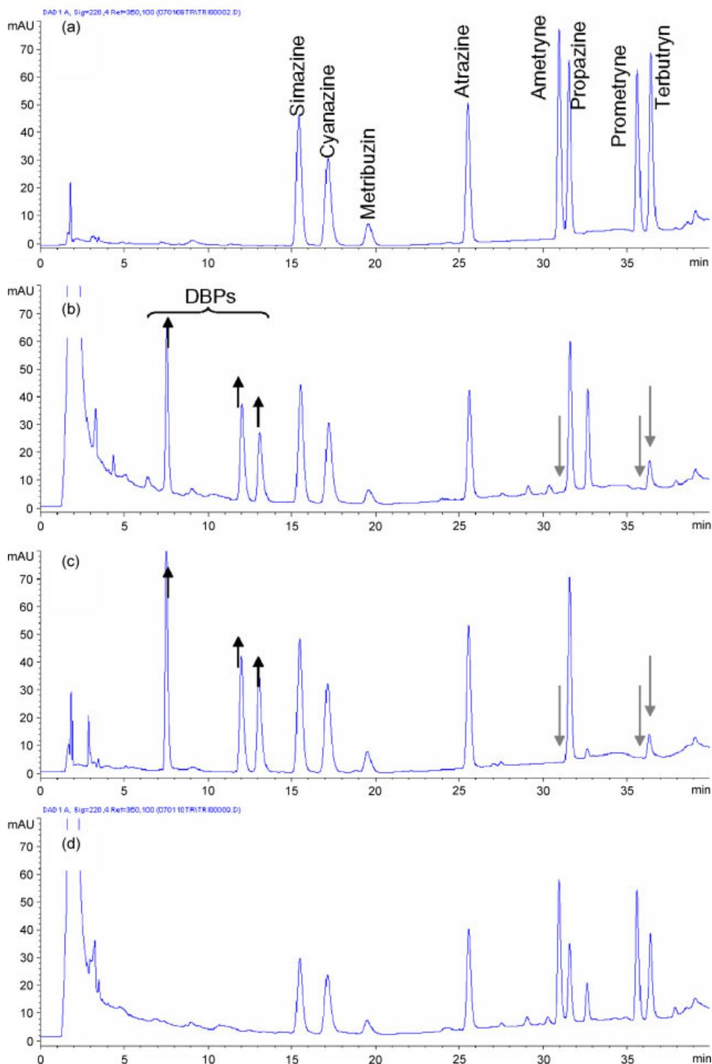
**Figure 2.** On-line SPE-LC-UV analysis of aqueous standard mixtures of the eight triazines (2  $\mu\text{g/l}$ ) prepared in (a) Milli-Q water, (b) tap water, (c) Milli-Q water spiked with 1 mg/l hypochlorite, and (d) tap water previously spiked with sodium sulphite.
