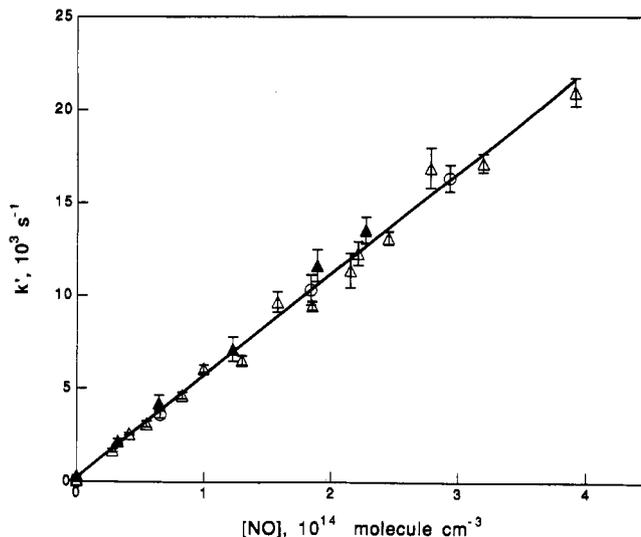
Figure 1. Plot of  $k'$  vs  $[\text{NO}]$  at  $T = 298$  K.  $\Delta$ ,  $P = 100$  Torr of He;  $\circ$ , 35 Torr of He;  $\blacktriangle$ , 20 Torr of He. The line is the linear least-squares fit to all of the data.
