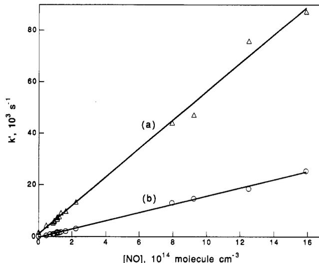
**Figure 3.** Plots of (a)  $k'_a$  and (b)  $k'_d$  vs  $[\text{NO}]$  obtained from the photolysis of  $\text{CF}_3\text{Br}$  ( $1.1 \times 10^{16}$  molecules  $\text{cm}^{-3}$ ),  $\text{O}_2$  (5 Torr) and NO. See text for description of  $k'_a$  and  $k'_d$ . These lines are linear least-squares fits.
