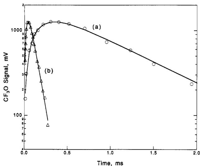
**Figure 2.**  $\text{CF}_3\text{O}$  temporal profiles following the 193-nm photolysis of  $\text{CF}_3\text{Br}$  ( $1.1 \times 10^{16}$  molecules  $\text{cm}^{-3}$ ),  $\text{O}_2$  (5 Torr) and NO: curves are (a)  $[\text{NO}] = 9.2 \times 10^{13}$  molecules  $\text{cm}^{-3}$  and (b)  $[\text{NO}] = 2.23 \times 10^{14}$  molecules  $\text{cm}^{-3}$ . The lines are fits to eq III.
