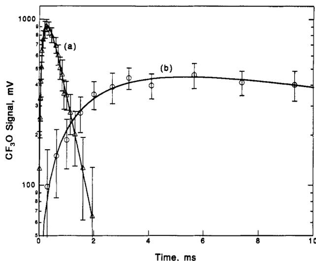
**Figure 7.** Back-to-back  $\text{CF}_3\text{O}$  temporal profiles from the 193-nm photolysis of  $\text{CF}_3\text{Br}$  ( $1.1 \times 10^{16}$  molecules  $\text{cm}^{-3}$ ) and  $\text{O}_2$  (5 Torr) with (a)  $[\text{NO}] = 1.04 \times 10^{14}$  molecules  $\text{cm}^{-3}$  and (b)  $[\text{O}_3] = 1.22 \times 10^{15}$  molecules  $\text{cm}^{-3}$ . Laser fluence was  $0.6 \text{ mJ pulse}^{-1} \text{ cm}^{-2}$ . The lines are nonlinear least-squares fit to eq III.
