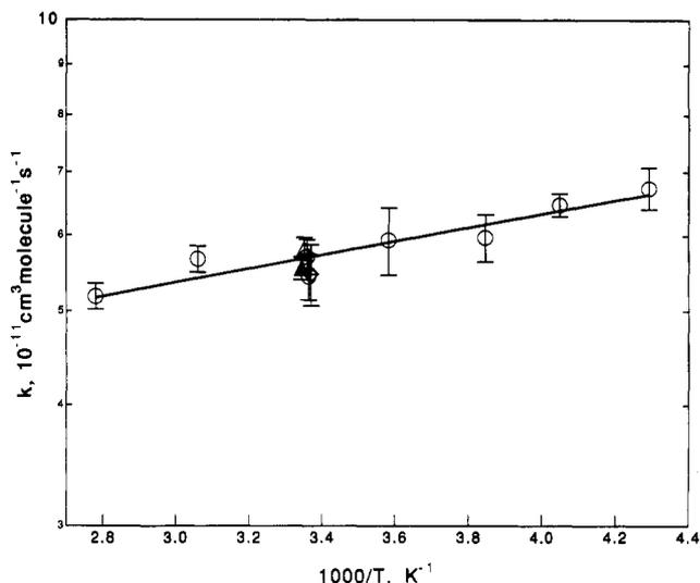
**Figure 4.** Observed rate coefficients for  $k_3$  vs  $1000/T$ .  $\circ$ ,  $P = 98$  and  $108$  Torr of He;  $\blacktriangle$ ,  $P = 35$  Torr of He;  $\triangle$ ,  $P = 20$  Torr of He;  $\diamond$ ,  $P = 70$  Torr of He and CF<sub>3</sub>O produced by CF<sub>3</sub>Br/O<sub>2</sub>/NO photolysis. The line is the least-squares fit to the data. Error bars are  $2\sigma$  and include only the experimental precision.
