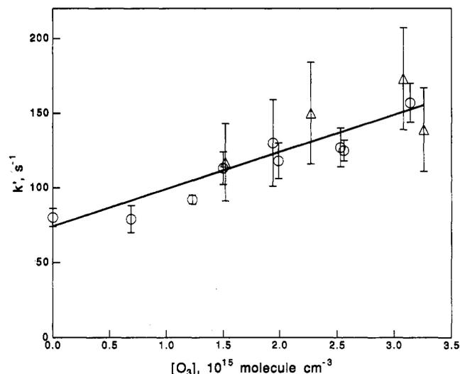
**Figure 6.** Plot of  $k'$  vs  $[\text{O}_3]$  at  $T = 298$  K. Conditions are [CF<sub>3</sub>OOCF<sub>3</sub>] =  $5 \times 10^{15}$  molecule cm<sup>-3</sup>;  $E = 0.27$  mJ pulse<sup>-1</sup> cm<sup>-2</sup>.  $\circ$ ,  $P = 100$  Torr of He;  $\triangle$ ,  $P = 100$  of He with 13 Torr of O<sub>2</sub> added.
