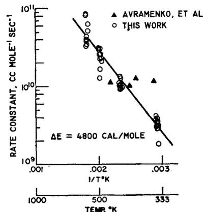
FIG. 4. Rate constants for O-atom disappearance by reaction with NH<sub>3</sub>.
