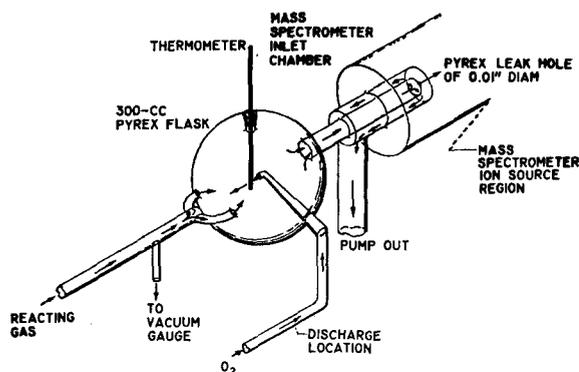
FIG. 1. Stirred reactor and connection to mass spectrometer.
