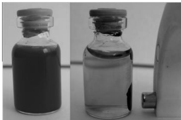
Figure 4. Response of the BAL-epoxy-M-support biocatalyst to the magnetic field.
