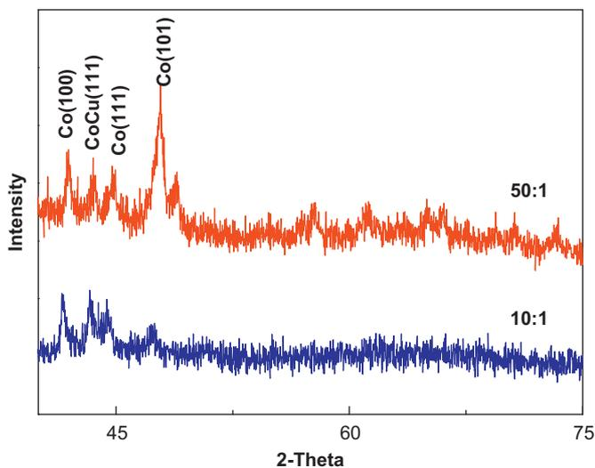
Fig. 2. (Color online) XRD pattern of as-synthesized Co–Cu nanowires with the deposited Co/Cu at the ratio of 50:1 and 10:1.
