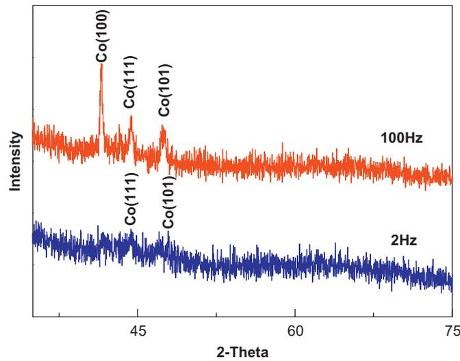
Fig. 4. (Color online) XRD pattern of nanowires wires with different supply frequency.
