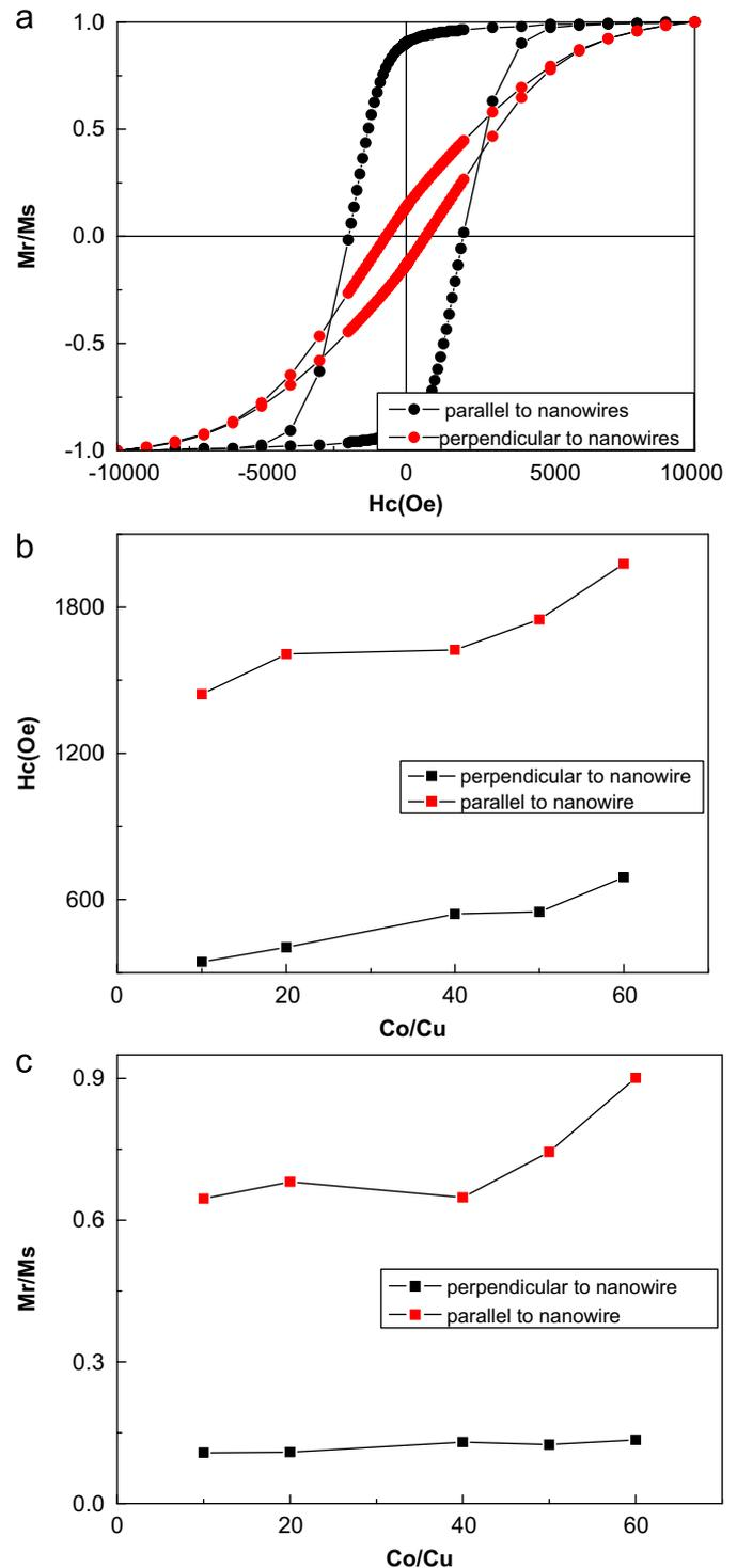
Fig. 3. (Color online) The typical hysteresis loop of the nanowires synthesized with Co/Cu ratio at 60:1 (a); the change in  $H_c$ ,  $H_{c\parallel}$  (b); and squareness ( $M_r/M_s$ ) (c) of the nanowires versus the Co/Cu ratio of the electrolyte.
