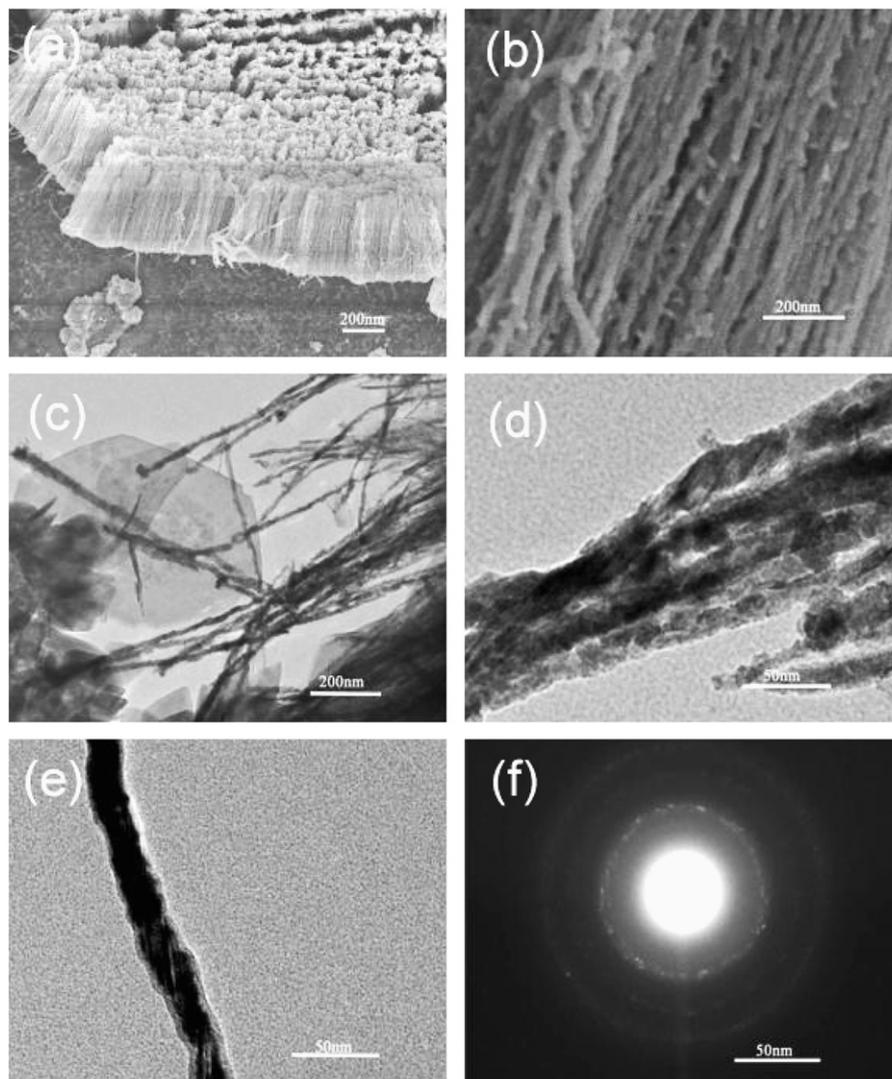
Fig. 1. FE-SEM images of Co–Cu nanowires (a, b); TEM images of Co–Cu nanowires (c, d, e, f).
