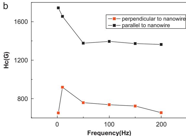
Fig. 5. (Color online) The typical hysteresis loops of the nanowires synthesized at the frequency of 2 Hz (a); and the variation tendency of  $H_c$  on frequency of electrodeposition (b).
