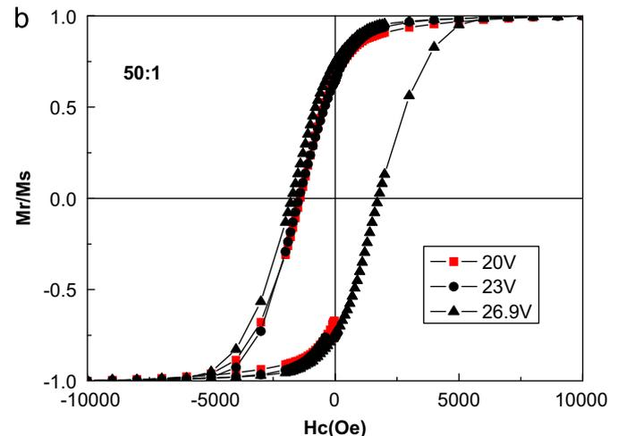
Fig. 6. (Color online) The hysteresis loops of the nanowires synthesized at different voltages at the electrolyte with different Co/Cu ratio.
