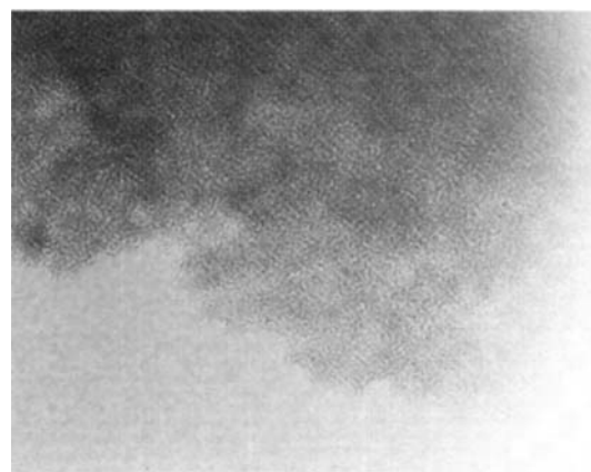
Fig. 2. TEM image of a calcined (773 K) MSU-1 alumina molecular sieve showing the regular wormlike channel motif, but no discernable long-range channel packing order. The material was prepared by using Tergitol 15-S-9 as the surfactant. The length of the bar corresponds to 60 nm.
