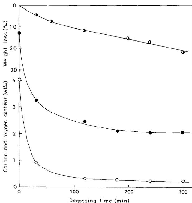
Fig. 4. The lowering of the carbon and oxygen contents and the change in weight of the sample during the isothermal degassing of vanadium in vacuum at 1600 °C: ○, oxygen; ●, carbon; ○, weight loss.
