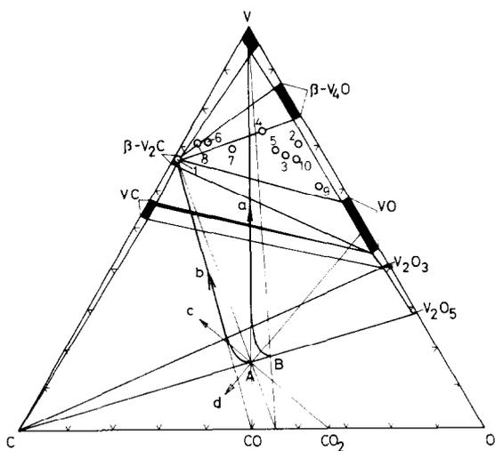
Fig. 2. A tentative V-C-O phase diagram at 1400 °C and the dissociation paths for the carbothermic reduction of  $V_2O_5$ .
