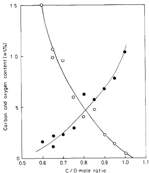
Fig. 3. The relationship between the C:O mole ratio in the starting material and the carbon and oxygen contents in the reduction products: ○, oxygen; ●, carbon.
