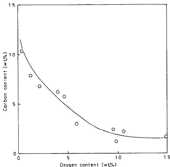
Fig. 1. Carbon and oxygen contents in the reduction products obtained by the carbothermic reduction in vacuum at 1400 °C.
