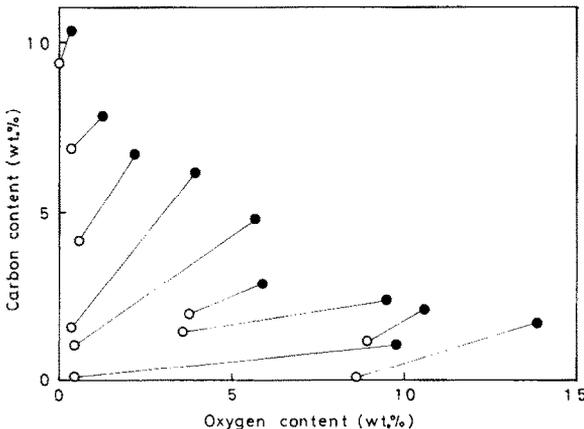
Fig. 8. Electron beam melting of the V–O binary alloys: ●, before melting; ○, after melting.
