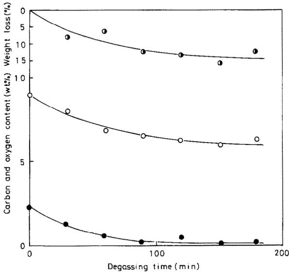
Fig. 5. The lowering of the carbon and oxygen contents and the change in weight of the sample during the isothermal degassing of vanadium at 1600 °C; ○, oxygen; ●, carbon; ○, weight loss.
