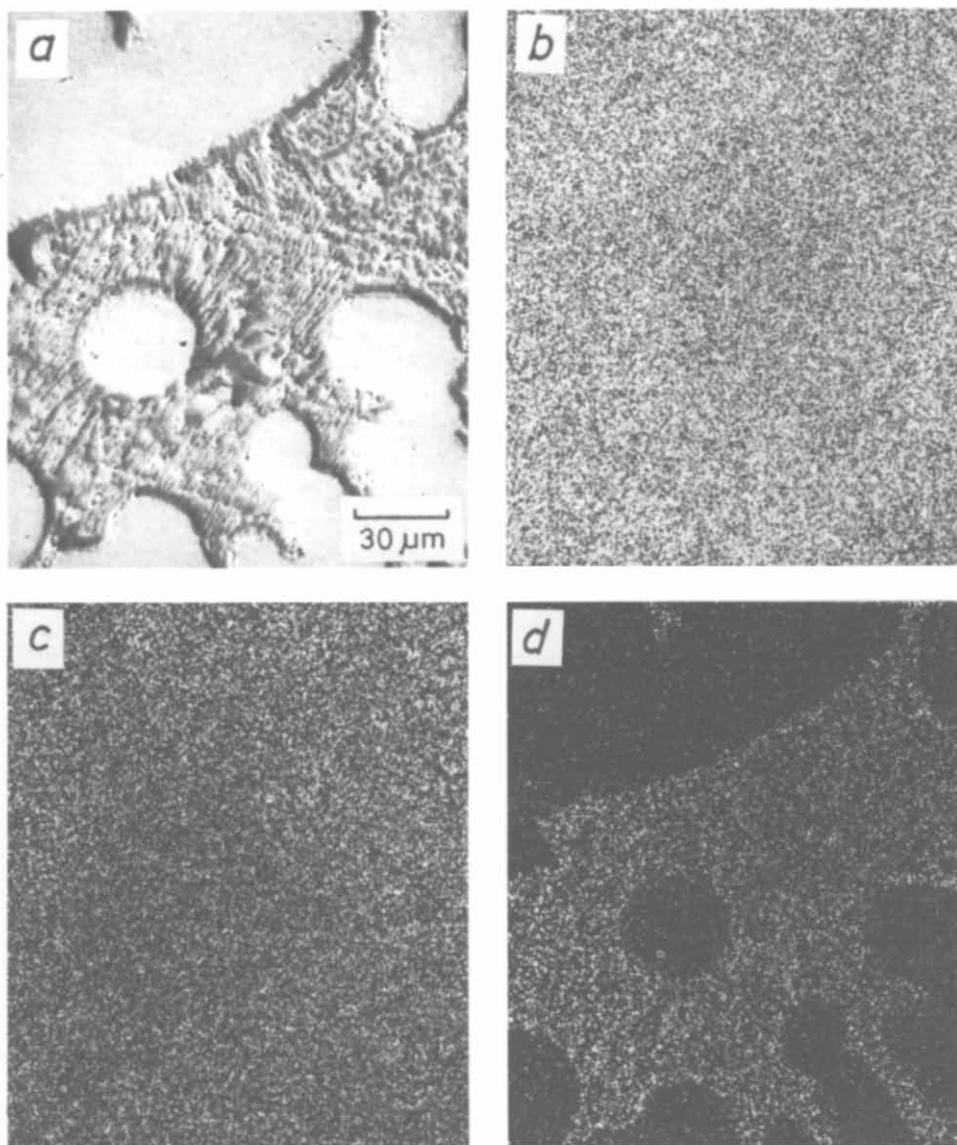
Fig. 7. Electron probe microanalysis of the V-0.6%C-0.5%O alloy melted by electron beam bombardment; (a) backscattered electron image; (b) vanadium map; (c) oxygen map; (d) carbon map.
