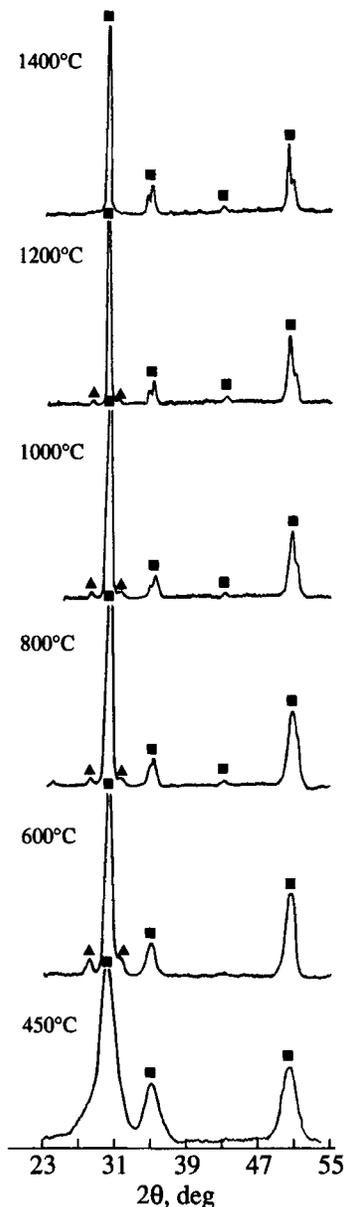
Fig. 2. XRD patterns of tetragonal  $(\text{ZrO}_2)_{0.97}(\text{Y}_2\text{O}_3)_{0.03}$  prepared from mechanically activated mixtures by firing between 450 and 1400°C.
