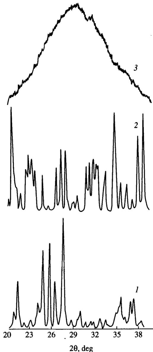
Fig. 1. XRD patterns of (1)  $\text{ZrO}(\text{NO}_3)_2 \cdot n\text{H}_2\text{O}$ , (2)  $\text{Y}(\text{NO}_3)_3 \cdot 6\text{H}_2\text{O}$ , and (3) their MA mixture ( $\text{ZrO}_2 : \text{Y}_2\text{O}_3 = 97 : 3$ ).
