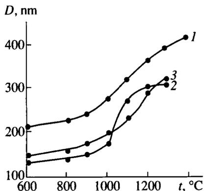
Fig. 3. Average particle size as a function of firing temperature for  $(\text{ZrO}_2)_{0.97}(\text{Y}_2\text{O}_3)_{0.03}$  materials prepared from starting mixtures mechanically activated in (1) air, (2) water, and (3) acetone.
