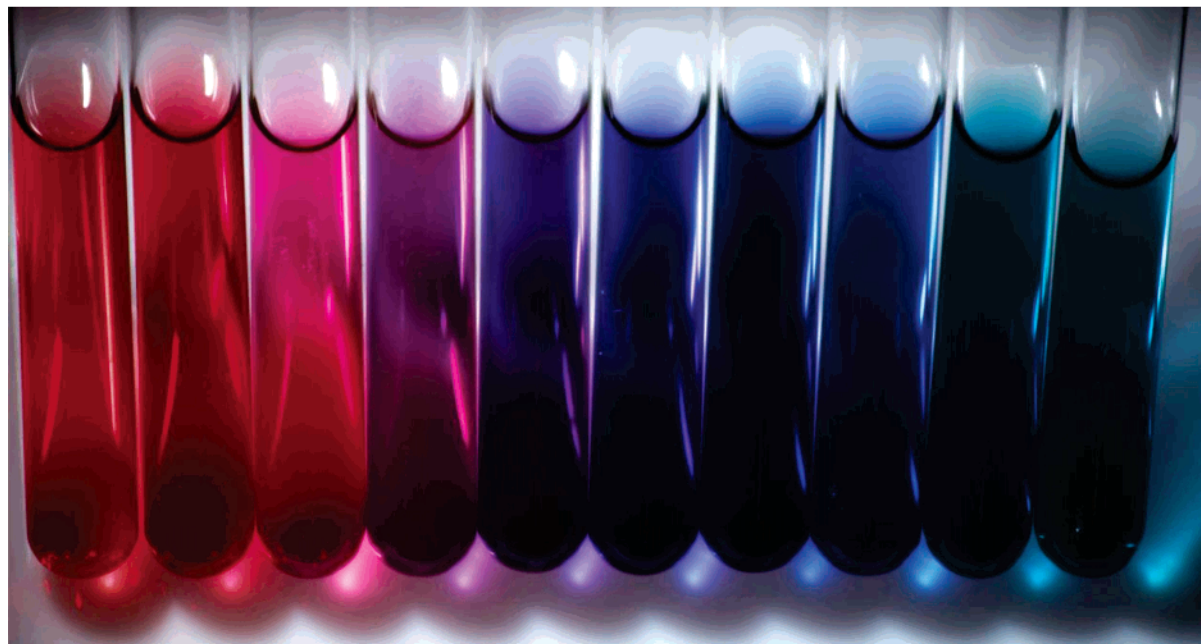
Figure 4. (a) UV-visible absorption spectra of nine HGN samples with varying diameters and wall thicknesses. (b) Image showing the color range of HGN solutions. The vial on the far left contains solid gold nanoparticles, the rest are HNGs with varying diameters and wall thicknesses.
