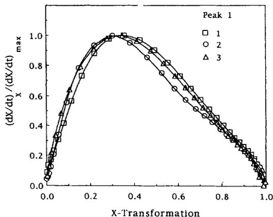
**Fig. 4** Normalized crystallization rate of the Al phase vs. fraction of Al crystallized for the three  $\text{Al}_{91}\text{La}_5\text{Ni}_4$  amorphous ribbons; curve 1 – soaked for 10 min at 1473 K followed by 5 min at 1373 K, curve 2 – soaked for 10 min at 1473 K followed by 5 min at 1273 K, curve 3 – soaked for 15 min at 1373 K
