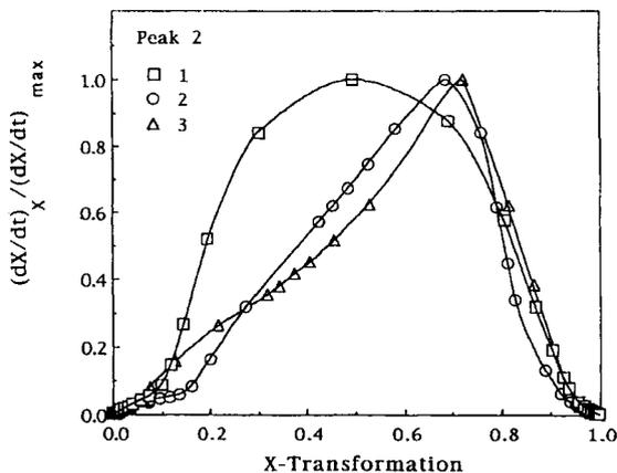
**Fig. 6** Normalized crystallization rate for  $\text{Al}_4\text{La}$  and  $\text{Al}_3\text{Ni}$  crystallization vs. fraction of both  $\text{Al}_4\text{La}$  and  $\text{Al}_3\text{Ni}$  crystallized for the three  $\text{Al}_{91}\text{La}_5\text{Ni}_4$  amorphous ribbons; curve 1 – soaked for 10 min at 1473 K followed by 5 min at 1373 K, curve 2 – soaked for 10 min at 1473 K followed by 5 min at 1273 K, curve 3 – soaked for 15 min at 1373 K
