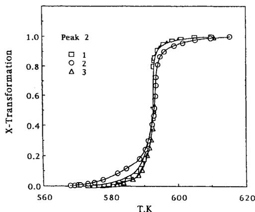
**Fig. 5** Fraction of  $\text{Al}_4\text{La}$  and  $\text{Al}_3\text{Ni}$  crystallized as a function of temperature/time for the three  $\text{Al}_{91}\text{La}_5\text{Ni}_4$  amorphous ribbons; curve 1 – soaked for 10 min at 1473 K followed by 5 min at 1373 K, curve 2 – soaked for 10 min at 1473 K followed by 5 min at 1273 K, curve 3 – soaked for 15 min at 1373 K
