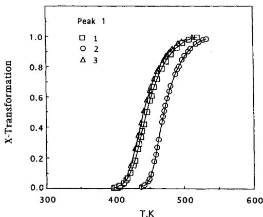
**Fig. 3** Fraction of Al crystallized as a function of temperature/time for the three  $\text{Al}_{91}\text{La}_5\text{Ni}_4$  amorphous ribbons; curve 1 – soaked for 10 min at 1473 K followed by 5 min at 1373 K, curve 2 – soaked for 10 min at 1473 K followed by 5 min at 1273 K, curve 3 – soaked for 15 min at 1373 K
