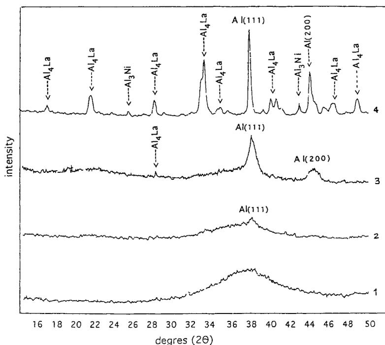
**Fig. 1** X-Ray diffractograms for Al<sub>91</sub>La<sub>5</sub>Ni<sub>4</sub> alloys. Curves 1, 2 and 3 represent specimens of ribbons 1, 2 and 3 before DSC analysis, respectively; curve 4 represents all three cases after DSC-analysis. Curve 1 – soaked for 10 min at 1473 K followed by 5 min at 1373 K, curve 2 – soaked for 10 min at 1473 K followed by 5 min at 1273 K, curve 3 – soaked for 15 min at 1373 K
