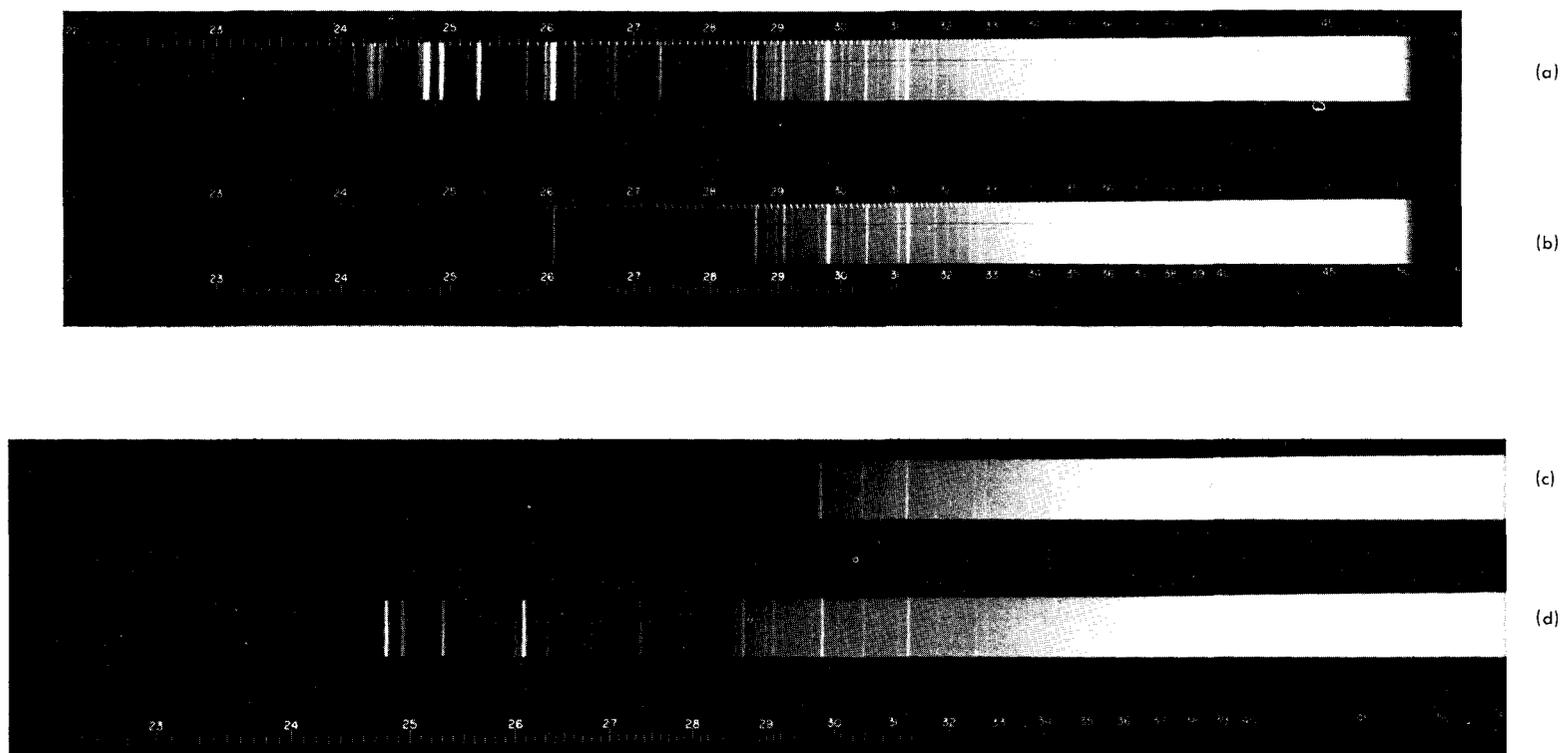
1. Flash absorption spectrograms behind incident shock waves. (a) Xenon flash lamp. (b) Shocked 1:2:100  $C_2F_4-NO-Ar$  gas mixture. (c) Shocked 1:100  $CF_4-Ar$  gas mixture. (d) Xenon flash lamp.
