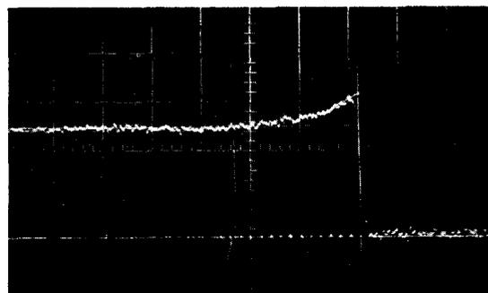
Fig. 2. Oscillogram record of  $CF_2$  uv absorption behind incident shock wave into 1:2:100  $C_2F_4$ - $NO$ -Ar gas mixture at 5.0 cm Hg initial pressure (Expt. No. 8). Shock temperature = 2080°K. Writing speed = 5  $\mu$ sec between vertical markers.
