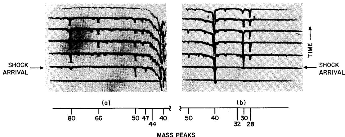
FIG. 3. Mass spectrogram of reflected-shock-heated 1:5:100  $C_2F_4$ -NO-Ar gas mixture. Analysis is performed at 25- $\mu$ sec intervals. Initial pressure=0.4 cm Hg. Reflected shock temperature $\approx$ 2600 $^\circ$ K.
