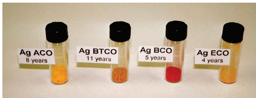
Figure 4. Vials with silver(I) cyanoximates showing the time of exposure to daylight.
