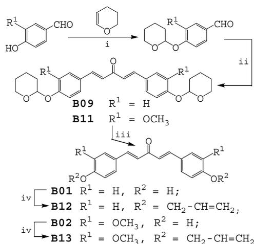
**Scheme 2.** Synthesis of presented compounds. Reagents and conditions: (i) pyridine–PTSA,  $\text{CH}_2\text{Cl}_2$ , rt; (ii)  $\text{CH}_3\text{COCH}_3$ ,  $\text{NaOH}/\text{EtOH}$ , rt; (iii) PTSA,  $\text{MeOH}$ , rt; (iv)  $\text{CH}_2=\text{CH}-\text{CH}_2\text{Br}$ ,  $\text{K}_2\text{CO}_3/\text{acetone}$ , reflux.
