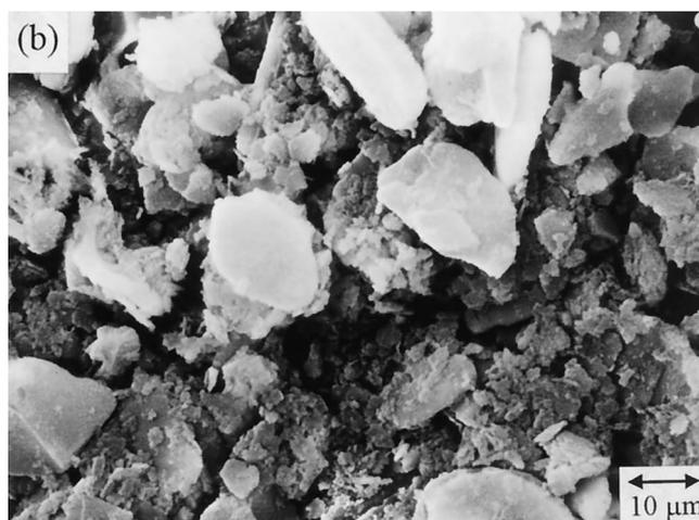
**Fig. 7.** SEM micrographs of (a) the conventionally treated (90°C, 240 min, and 1M H<sub>2</sub>SO<sub>4</sub>) sample and (b) the microwave-treated (90°C, 120 min, and 1M H<sub>2</sub>SO<sub>4</sub>) sample obtained by calcining at 1000°C for 1 h.
