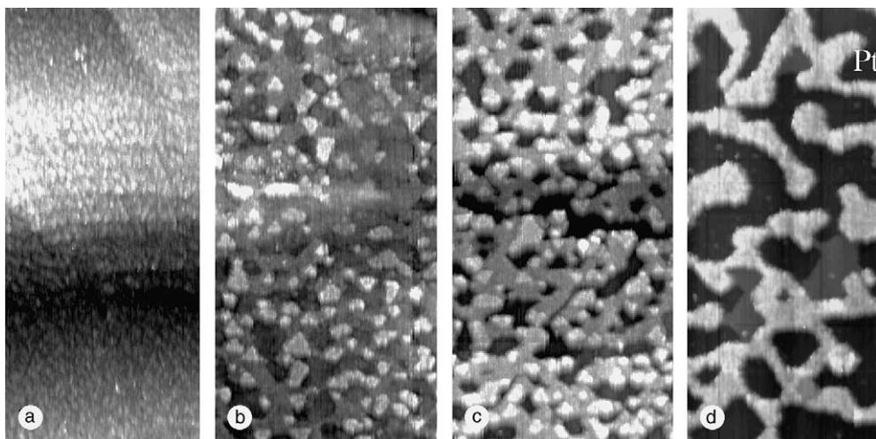
Fig. 1. STM images of 4 ML thick  $\text{ZrO}_2$  films on Pt(111) deposited at room temperature taken after deposition (a) and after postannealing at 1000 K (b) (annealing time 20 s) and 1050 K (c,d; annealing time 20 and 60 s, respectively). Image size 75 nm  $\times$  150 nm.
