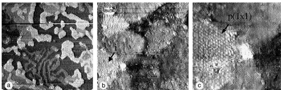
Fig. 3. STM images of continuous and smooth  $\text{ZrO}_2$  film on  $\text{Pt}(1\ 1\ 1)$ . Mean thickness 4 ML. 470 K deposition, postannealing at 950 K. Image size 100 nm  $\times$  100 nm (a), 20 nm  $\times$  20 nm (b), and 8 nm  $\times$  8 nm (c). For explanation see text.
