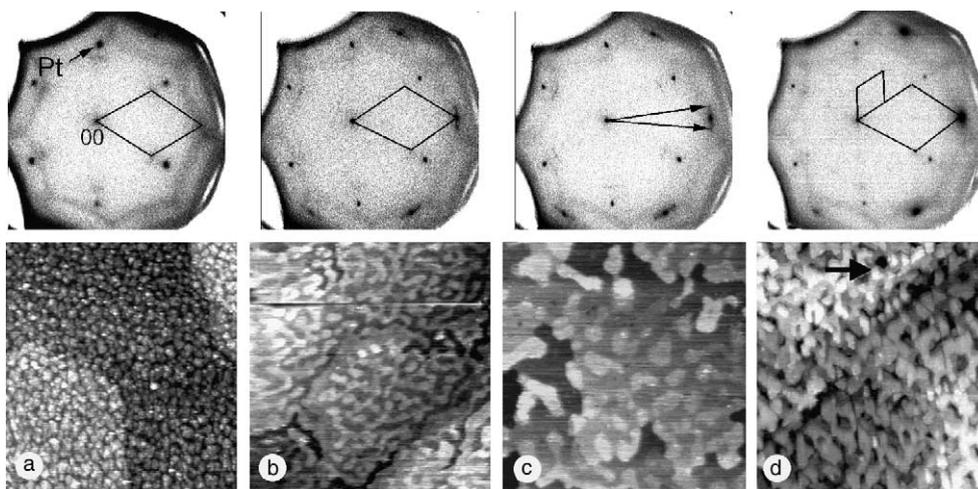
Fig. 2. STM images and LEED patterns of 4 ML thick  $\text{ZrO}_2$  films on Pt(111) deposited at 470 K taken after deposition (a) and after postannealing at 950 K (b,c; annealing time 10 and 20 min, respectively) and 1020 K (annealing time 20 min). Image size 150 nm  $\times$  150 nm. LEED energy 66 eV. In the LEED patterns the unit cells of the  $p(1 \times 1)$  and  $p(2 \times 2)$  structures are indicated.
