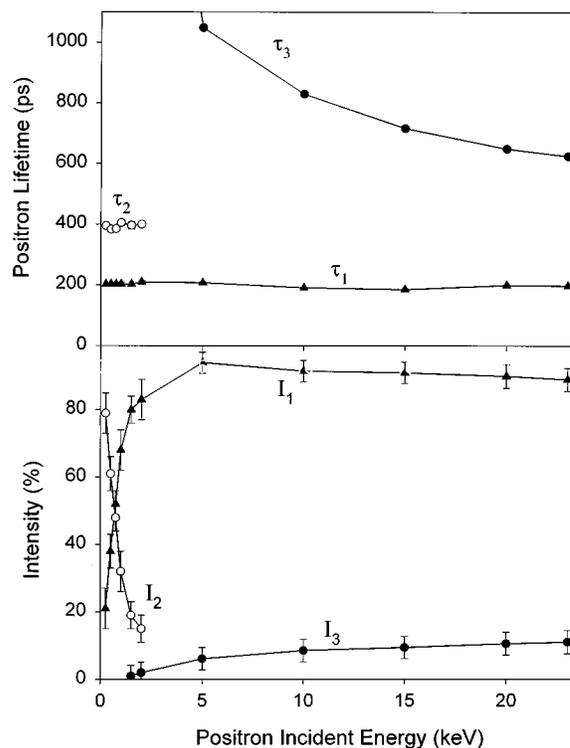
FIG. 2. (a) Positron lifetimes and (b) related intensities for thermally grown alumina scale on iron aluminide substrate as a function of positron energy. For lower energies ( $<2$  keV),  $I_2$ ,  $I_3$ ,  $\tau_2$  and  $\tau_3$  were determined by fitting (POSFIT) with  $\tau_1$  fixed at the average bulk lifetime (202.5 ps). For other energies, all parameters were obtained by fitting.
