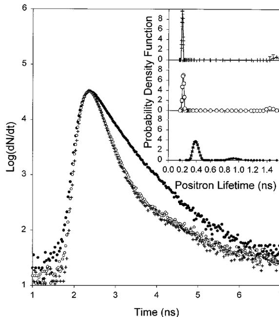
FIG. 1. Semi-log plots of the counting rates as functions of the arrival time of annihilation gamma rays for the thermally grown Al<sub>2</sub>O<sub>3</sub> scales on both Fe<sub>3</sub>Al+Y<sub>2</sub>O<sub>3</sub> (open circles) and β-NiAl+Hf (crosses), and for the PVD Al<sub>2</sub>O<sub>3</sub> film on Fe<sub>3</sub>Al+Zr (filled circles). Inset: Probability density functions as a function of positron lifetime, resulting from Laplace inversion (CONTIN).
