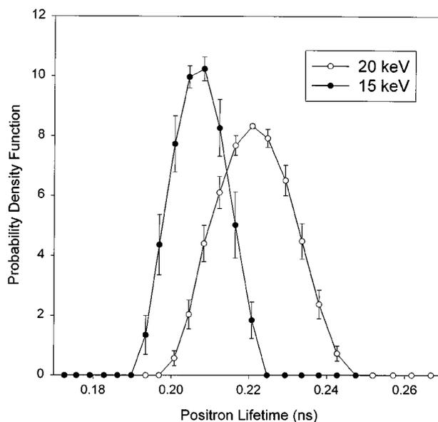
FIG. 3. Probability density functions as a function of positron lifetime for 15 and 20 keV positrons ejected into the thermally grown  $\text{Al}_2\text{O}_3$  scale on the iron-aluminide substrate.
