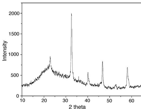
Fig. 3. X-ray diffraction spectra of  $\text{LaMnO}_{3+\delta}$  nanowire array embedded in the AAM template.
