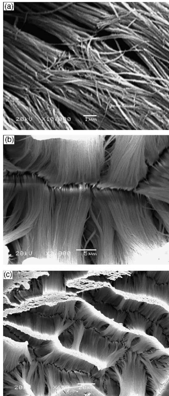
Fig. 2. SEM images of  $\text{LaMnO}_{3+\delta}$  nanowire array: (a) cross-section view, (b) top view in low magnification, and (c) top view in high magnification.
