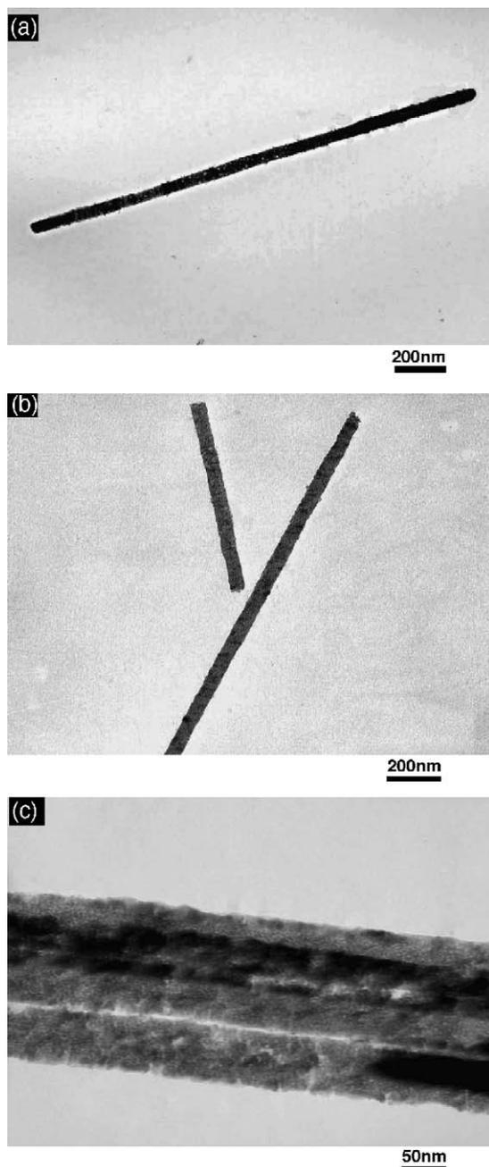
Fig. 1. TEM photographs: (a and b) freestanding  $\text{LaMnO}_{3+\delta}$  nanowires and (c) parallel  $\text{LaMnO}_{3+\delta}$  nanowire array.
