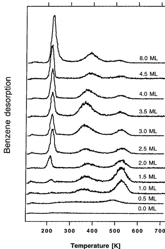
**Figure 2.** Desorption of benzene ( $m/e = 78$ ) following a 70 langmuir acetylene exposure at 150 K for various Pd loadings as indicated.
