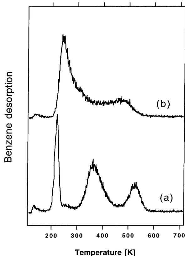
**Figure 4.** Benzene ( $m/e = 78$ ) desorption following (a) initial and (b) repeated adsorption of 70 langmuirs of C<sub>2</sub>H<sub>2</sub> at 150 K on Pd particles ( $\sim 50$  Å).
