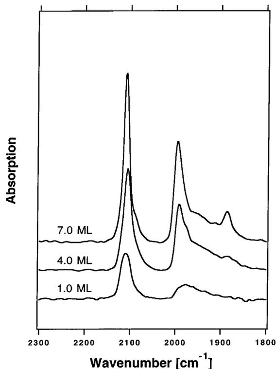
**Figure 1.** IRA spectra of CO chemisorbed on alumina thin film supported Pd particles corresponding to deposition of 1, 4, and 7 ML of Pd. All spectra are obtained at 110 K in  $1.5 \times 10^{-6}$  Torr CO.
