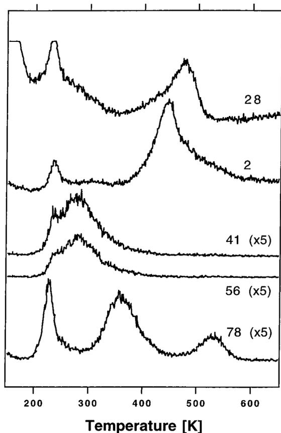
**Figure 3.** Mass fragments  $m/e = 2, 28, 41, 56,$  and  $78$  detected in TPD following a 70 langmuir acetylene exposure at 150 K on particles corresponding to 3 ML of Pd ( $\sim 50$  Å).
