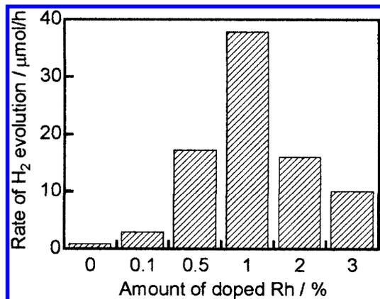
**Figure 2.** Dependence of H<sub>2</sub> evolution activity of Rh-doped SrTiO<sub>3</sub> upon the doping amount. Catalyst, 0.3 g; cocatalyst, Pt (0.5 wt %); reactant solution, 150 mL of 10 vol % aqueous MeOH; light source, 300 W Xe lamp with cutoff filters ( $\lambda > 440$  nm).
