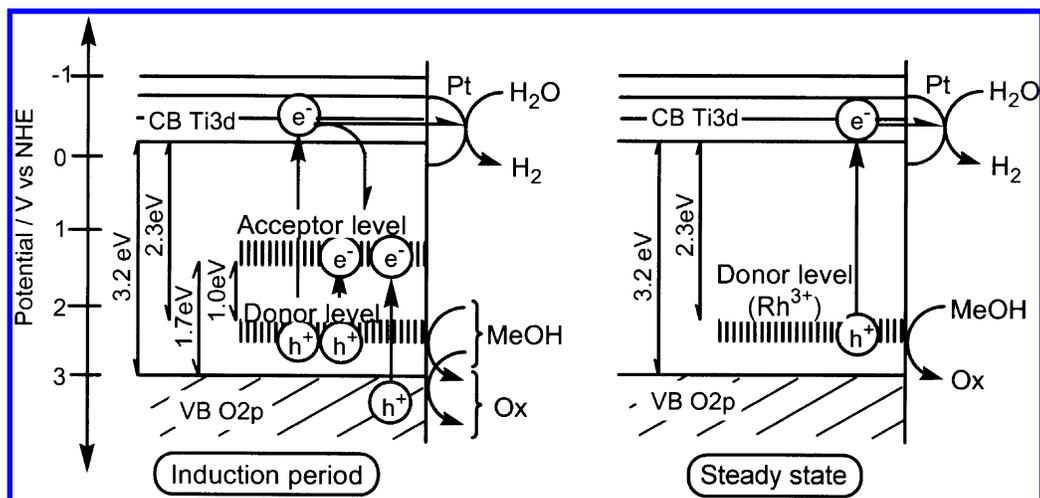
**Figure 5.** Proposed band structure and visible light response of Rh-doped SrTiO<sub>3</sub> photocatalyst.
