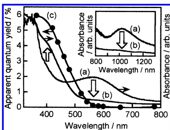
**Figure 4.** Diffuse reflectance spectra of (a) before and (b) after photocatalytic reaction, and (c) action spectrum for H<sub>2</sub> evolution from an aqueous methanol solution over a SrTiO<sub>3</sub>:Rh(1%) photocatalyst. The inset shows an expanded view of the spectra in the wavelength region from 800 to 1300 nm. Catalyst, 0.3 g; cocatalyst, Pt (0.1 wt %); reactant solution, 150 mL of 10 vol % aqueous methanol solution; light source, 300 W Xe lamp.
