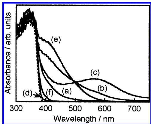
**Figure 1.** Diffuse reflectance spectra of SrTiO<sub>3</sub>:M(0.5%). M = (a) Mn, (b) Ru, (c) Rh, (d) Pd, (e) Ir, and (f) Pt. A broken line represents a spectrum of nondoped SrTiO<sub>3</sub>.
