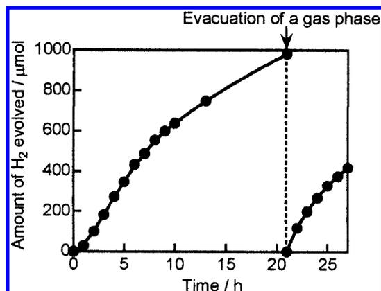
**Figure 3.** H<sub>2</sub> evolution from an aqueous methanol solution under visible light irradiation over a Pt(0.1 wt %)/SrTiO<sub>3</sub>:Rh(1%) photocatalyst prepared by solid-state reaction at 1273 K for 10 h. Catalyst, 0.3 g; reactant solution, 150 mL of 10 vol % aqueous MeOH; light source, 300 W Xe lamp with cutoff filters ( $\lambda > 440$  nm).
