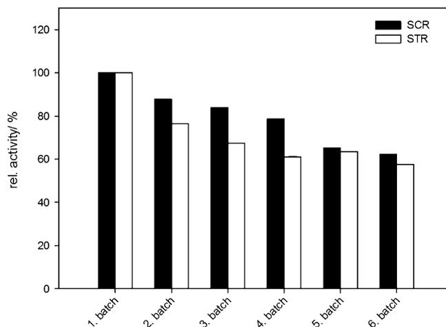
**Figure 6.** Recycling study with immobilized lipase CAL-B (2 h per batch) in the SCR and the STR; 100% relative activity refers to 33% (SCR) and 39% conversions (STR) of (*R,S*)-1-phenylethanol in the first batch.
