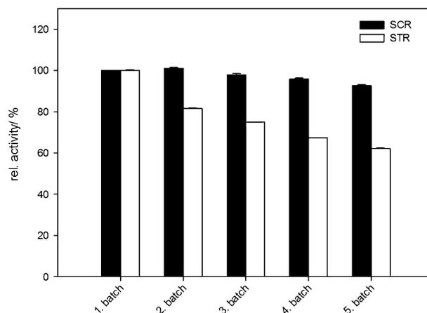
**Figure 5.** Recycling study with immobilized GibZea (*R*)-transaminase (2 h per batch) in the SCR and the STR; 100% relative activity refers to 19% conversion of (*R*)-1-phenylethylamine in the first batch.
