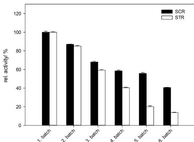
**Figure 7.** Recycling study with encapsulated resting *E. coli* cells that expressed the CHMO in the SCR and the STR (2 h per batch); 100% relative activity refers to 7.5% conversion of cyclohexanone in the first batch.
