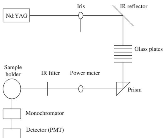
Fig. 5. Schematic arrangement of the experimental setup used for measuring the SHG efficiency.
