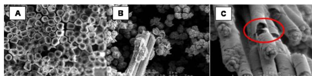
Figure 6. (Color online) SEM micrographs for Pt electrochemically deposited through an AAO membrane at -0.15 V in a 0.5 \text{ mM Na}_2\text{PtCl}_6 , KCl-free plating bath. (A) Electrode removed immediately from the electroplating solution and rinsed with deionized water. [(B) and (C)] Electrode left for 5 h in the electroplating solution under OCP.
