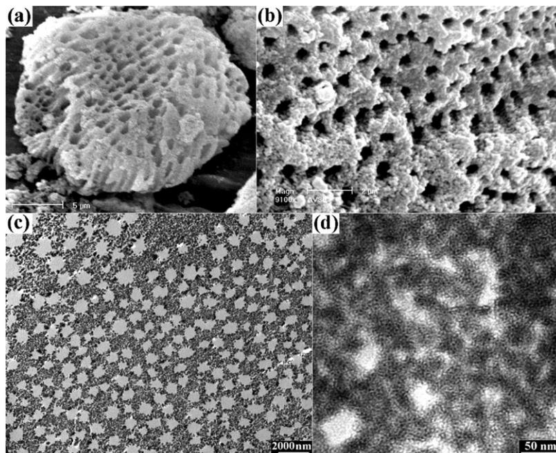
**Fig. 1** (a, b) SEM images of the synthesised zirconia particles showing uniform macroporosity; (c) low-magnification TEM image of a cross-section of the synthesised zirconia showing the uniform macropore structure with mesopores in the walls; (d) high-magnification TEM image of a region of the macropore walls, showing the assembly of zirconia nanoparticles into wormhole-like supermicropores with irregular mesovoids.
