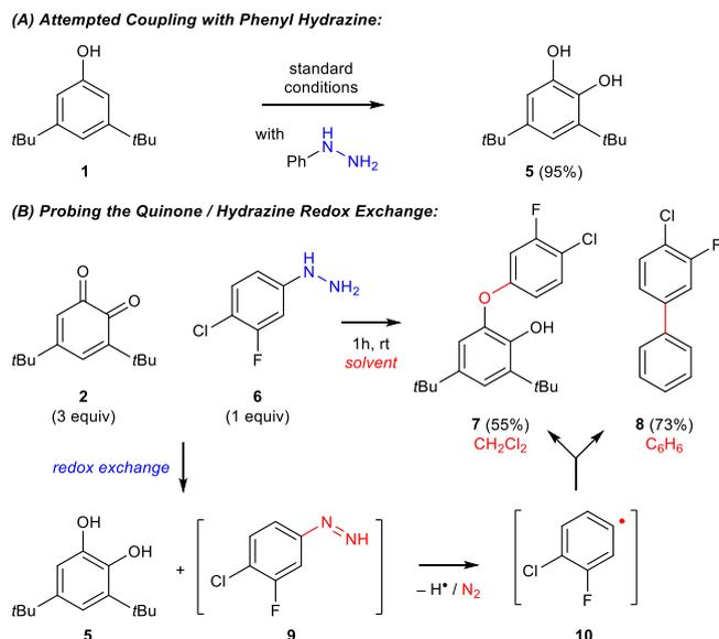
**Scheme 4.** (A) Redox reaction of **1** with phenylhydrazine. (B) Mechanistic studies on quinone / hydrazine redox exchange.
