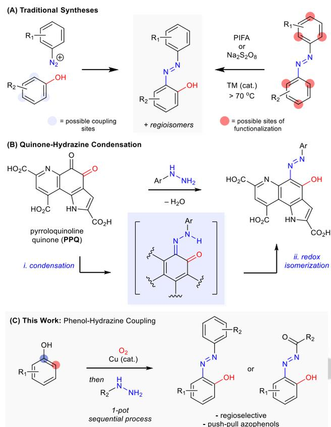
**Scheme 2.** (A) Classical syntheses by diazo coupling, and transition metal catalyzed hydroxylation. (B) PQQ and hydrazine condensation. (C) Work described therein.
