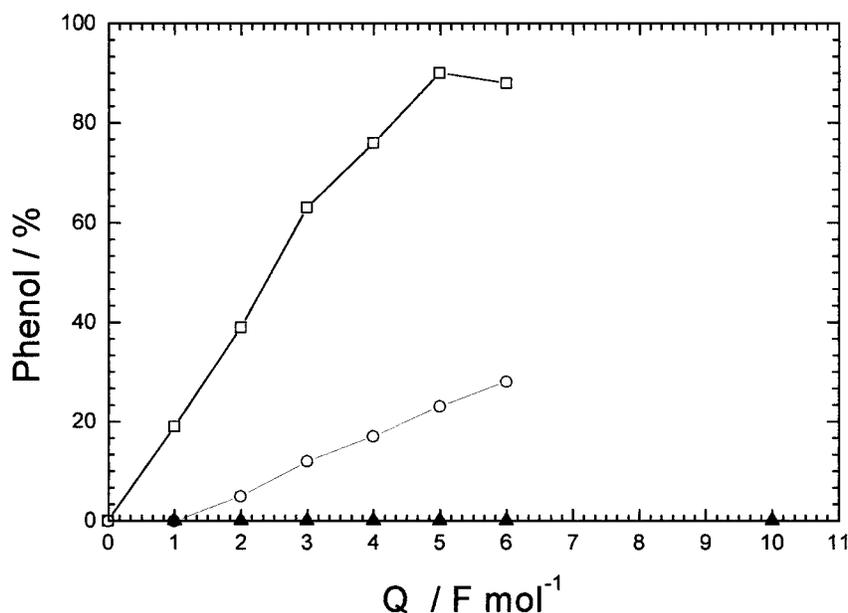
FIGURE 2. Yield of phenol formed in the electrolysis of 4-chlorophenol (□), 2,6-dichlorophenol (○), and PCP (▲) on a RVC electrode under galvanostatic conditions ( $i = 25$  mA) in 1 M NaOH at 50 °C.
