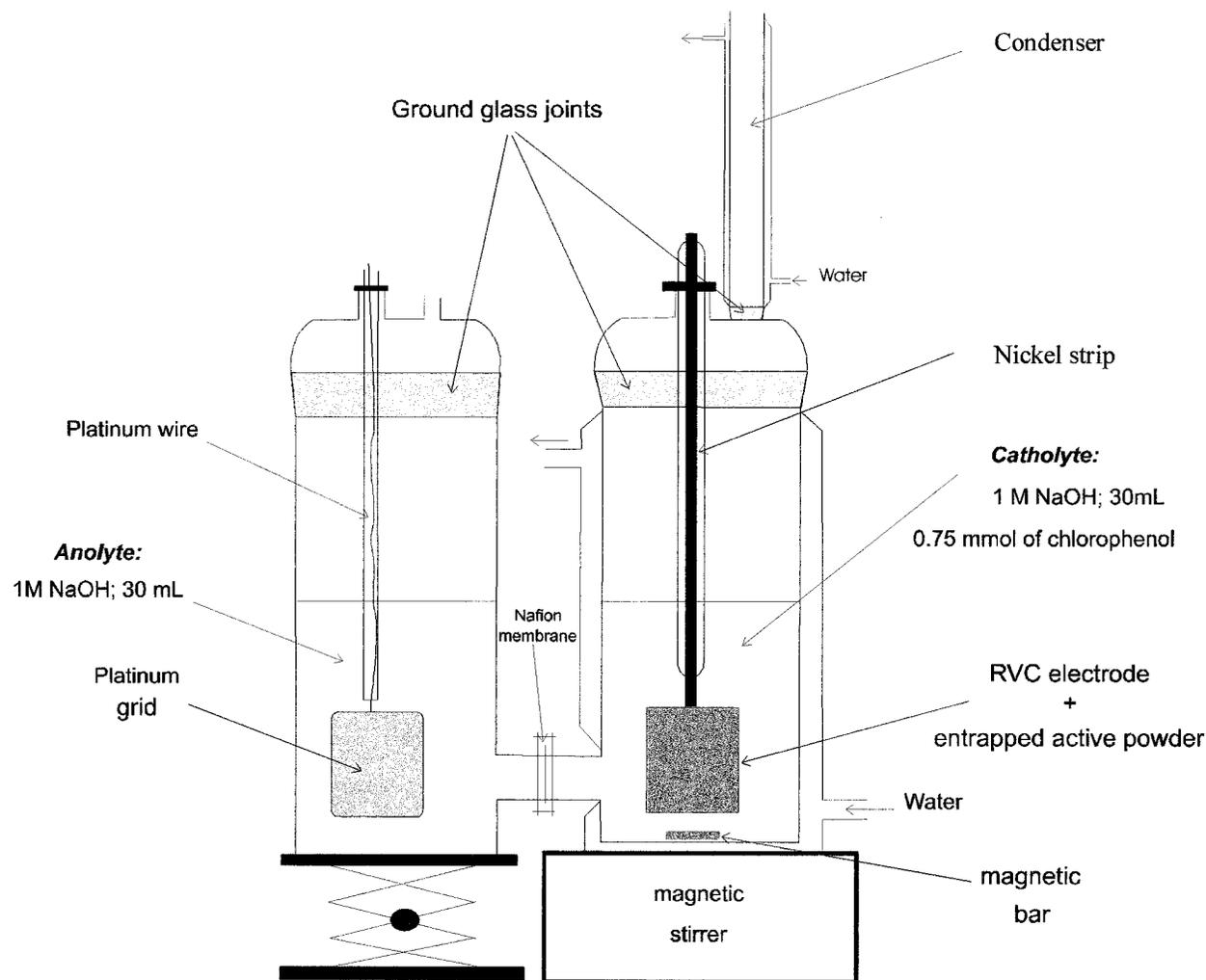
FIGURE 1. Two-compartment cell used for the electrolyses.
