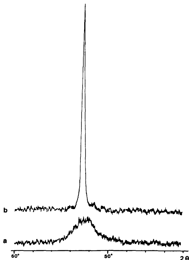
Fig. 3. Strongest reflection in the diffractogram of an Fe/Co alloy (Table 5, No. 3). (a) Untreated original sample. (b) After 2 h at 400 °C (CoK \alpha -irradiation with Fe filter).
