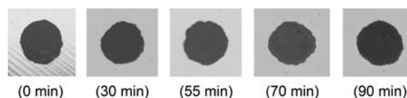
Figure 5. Photographs of the PAA thin film anodized for 175 s with different etching times from 0 to 90 min.
