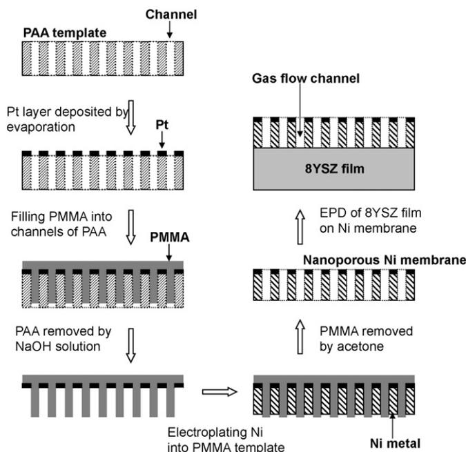
Fig. 1. Schematic representation of using two-step replication technique to fabricate nanoporous Ni membrane and 8YSZ/Ni membrane structure.
