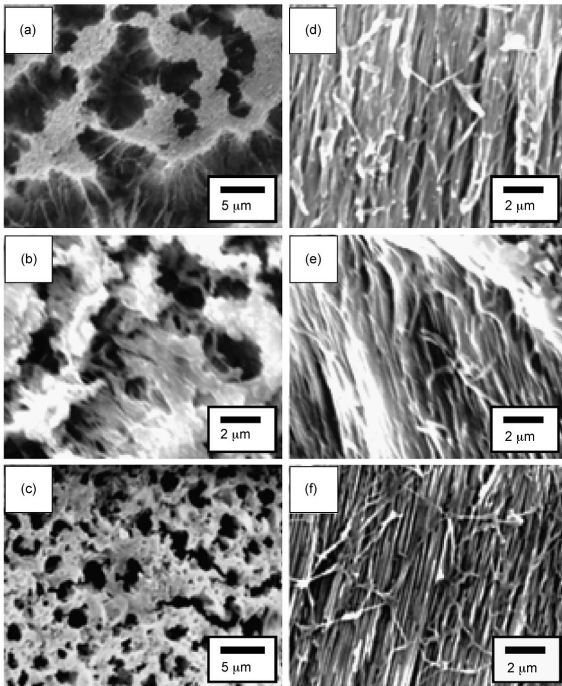
Fig. 4. Top-view images of PMMA nano-arrays fabricated at PMMA concentration of: (a) 10 wt%, (b) 13 wt%, (c) 15 wt%, cross-section images (d) 10 wt%, (e) 13 wt%, and (f) 15 wt% (PMMA  $M_w = 965,000$  g/mol).
