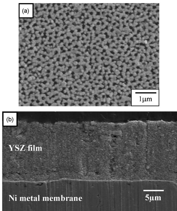
Fig. 6. (a) SEM top-view observation of Ni membrane fabricated by electroplating. (b) SEM cross-sectional image of 8YSZ film deposited on Ni membrane by EPD.
