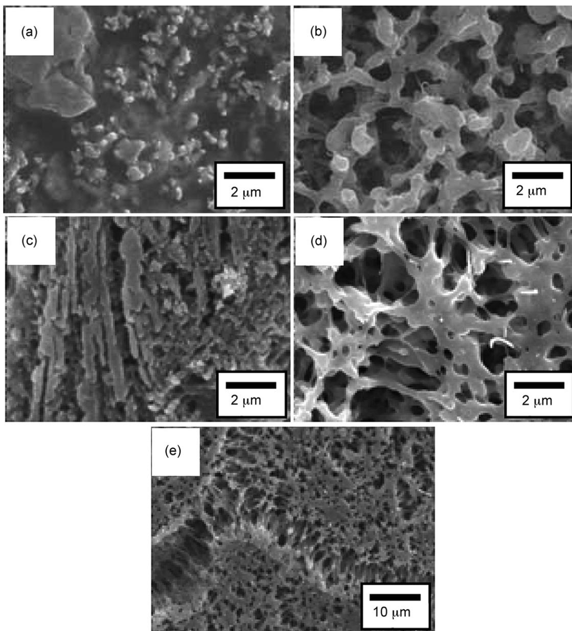
Fig. 3. SEM top-views of replicated negative type of PMMA ( $M_w = 15,000$  g/mol) that fabricated with various concentrations: (a) 10 wt% and (b) 15 wt%. SEM top-views of replicated negative-type structures of PMMA ( $M_w = 70,000$  g/mol) that fabricated with various concentrations: (c) 10 wt% and (d) and (e) 15 wt%.
