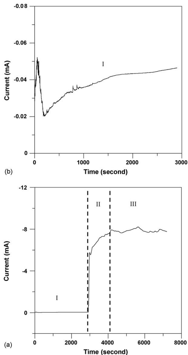
Fig. 5. The current transient curves for (a) long time and (b) short time (<3000 s) of Ni metal electroplating into the negative-type PMMA.
