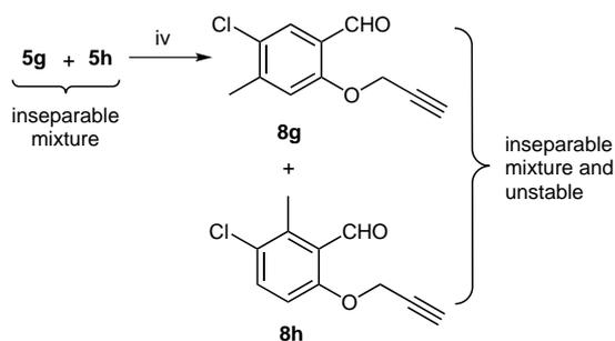
**Scheme 1** Reagents and conditions: (i) (when R<sup>5</sup> = Me, Et): K<sub>2</sub>CO<sub>3</sub>, reflux, 10–12 h; (ii) (when R<sup>5</sup> = aryl): KOH, MeOH, r.t., 2–3 h, then 4 N HCl; (iii) propargyl bromide, anhyd K<sub>2</sub>CO<sub>3</sub>, NaI (cat.), dry acetone, reflux, 5–6 h; (iv) propargyl bromide, anhyd K<sub>2</sub>CO<sub>3</sub>, NaI (cat.), dry MeCN, reflux, 2 h.
