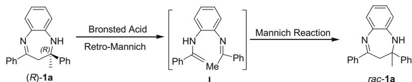
**Scheme 1.** Explanation of the dynamic kinetic transfer hydrogenation.
