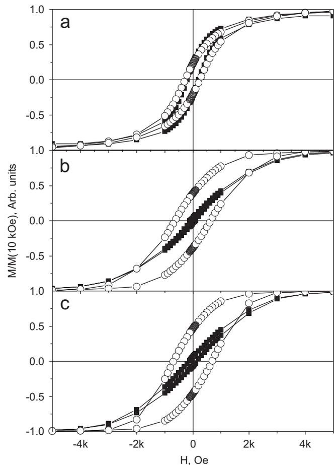
Fig. 2. Hysteresis loops for nickel: (a) nanodots, (b) nanorods and (c) nanowires measured at 5 K with the field applied parallel (—■—) and perpendicular (---○---) to the membrane plane.
