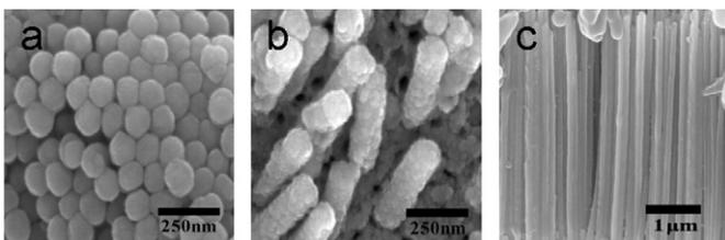
Fig. 1. The FE-SEM images of nickel: (a) nanodots, (b) nanorods and (c) nanowires after removal of the AAO templates. The diameter, length and the distance between the pores of the AAO template are 100 nm, 40 μm, and 210 nm, respectively.
