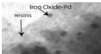
FIGURE 2. TEM micrograph of Iron Oxide-Pd (12 nm) encapsulated inside a solvent-swollen polystyrene solid-phase bead (partial). The swollen polystyrene polymers were deposited at the edge of a hole on a lacey TEM grid for improved imaging contrasts.
