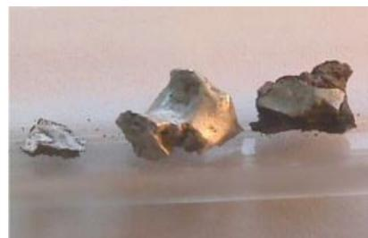
Figure 7. Fragments of a tin sponge. The diameters of the two bigger pieces are around 2 to 3 mm.
