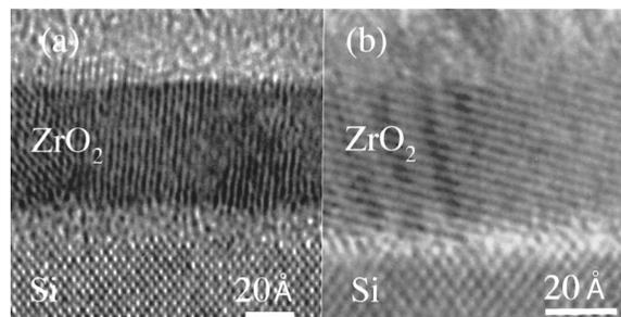
FIG. 1. Cross-sectional TEM micrographs show the morphology of the TiN/ $\text{ZrO}_2$ / $p$ -Si gate stack structure on (a) chemical oxide-terminated silicon and (b) HF-last silicon.
