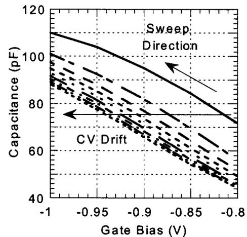
FIG. 5. Ten successive  $\pm 2$  V sweeps show monotonic flatband shift (reverse sweeps not shown).
