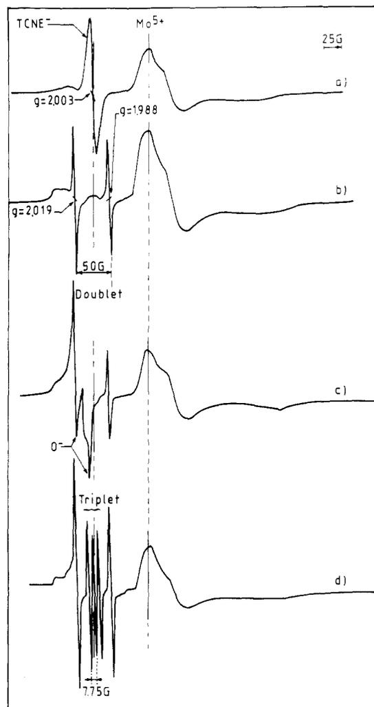
**Figure 1.** EPR spectra of the grafted Mo/SiO<sub>2</sub> catalyst, obtained after TCNE adsorption in the following conditions: after H<sub>2</sub> reduction (a); after O<sup>-</sup> formation: the O<sup>-</sup> signal is no more visible (b), and the O<sup>-</sup> signal is still visible (c); after D<sub>2</sub> reduction and O<sup>-</sup> formation (d). All the species were recorded at room temperature.
