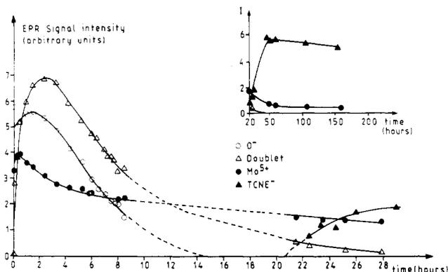
**Figure 2.** Evolution of the signal intensities of the different species visible in the EPR spectrum when TCNE was adsorbed on the reduced Mo/SiO<sub>2</sub> catalyst containing O<sup>-</sup> ions (the intensities were measured from the height of each signal; they are expressed in arbitrary units).
