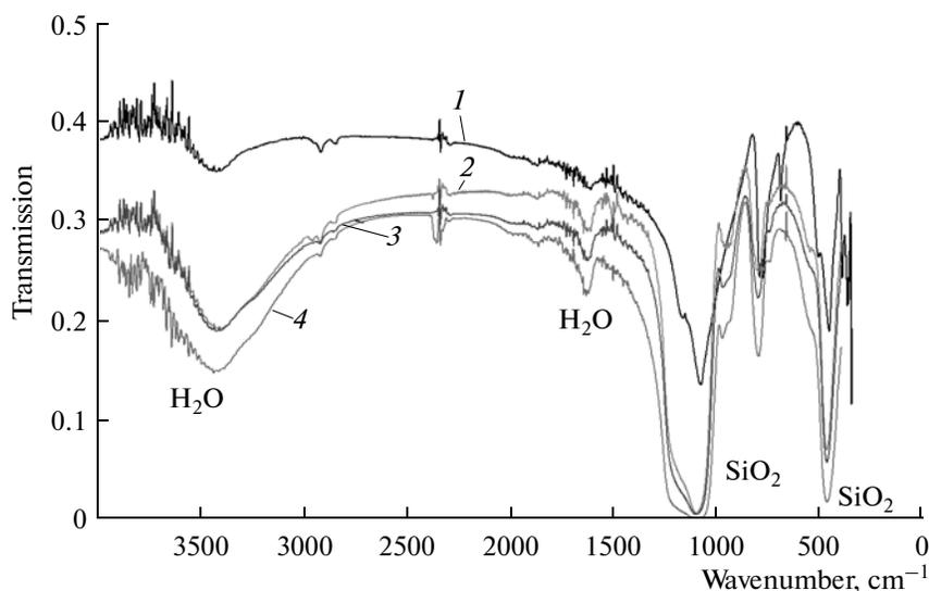
**Fig. 4.** IR spectra of the (1) quartz sand and (2–4) amorphous silica powders prepared at 80°C. The initial (NH<sub>4</sub>)<sub>2</sub>SiF<sub>6</sub> content of aqueous solution was (2) 33, (3) 20, and (4) 3 wt %.
