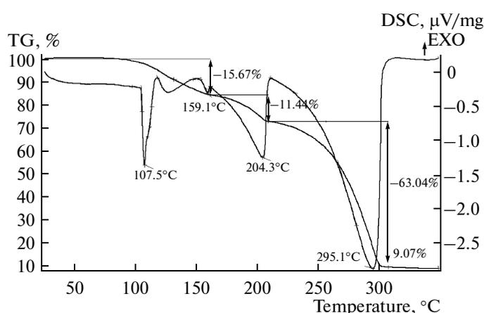
**Fig. 1.** DSC and TG curves for the reaction between quartz sand and ammonium bifluoride.
