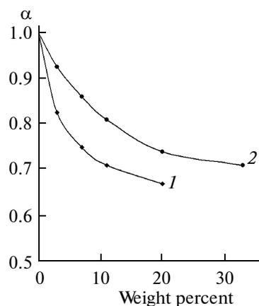
**Fig. 2.** Degree of extraction of amorphous silica against initial ammonium hexafluorosilicate concentration in aqueous solution at (1) 25 and (2) 80°C.
