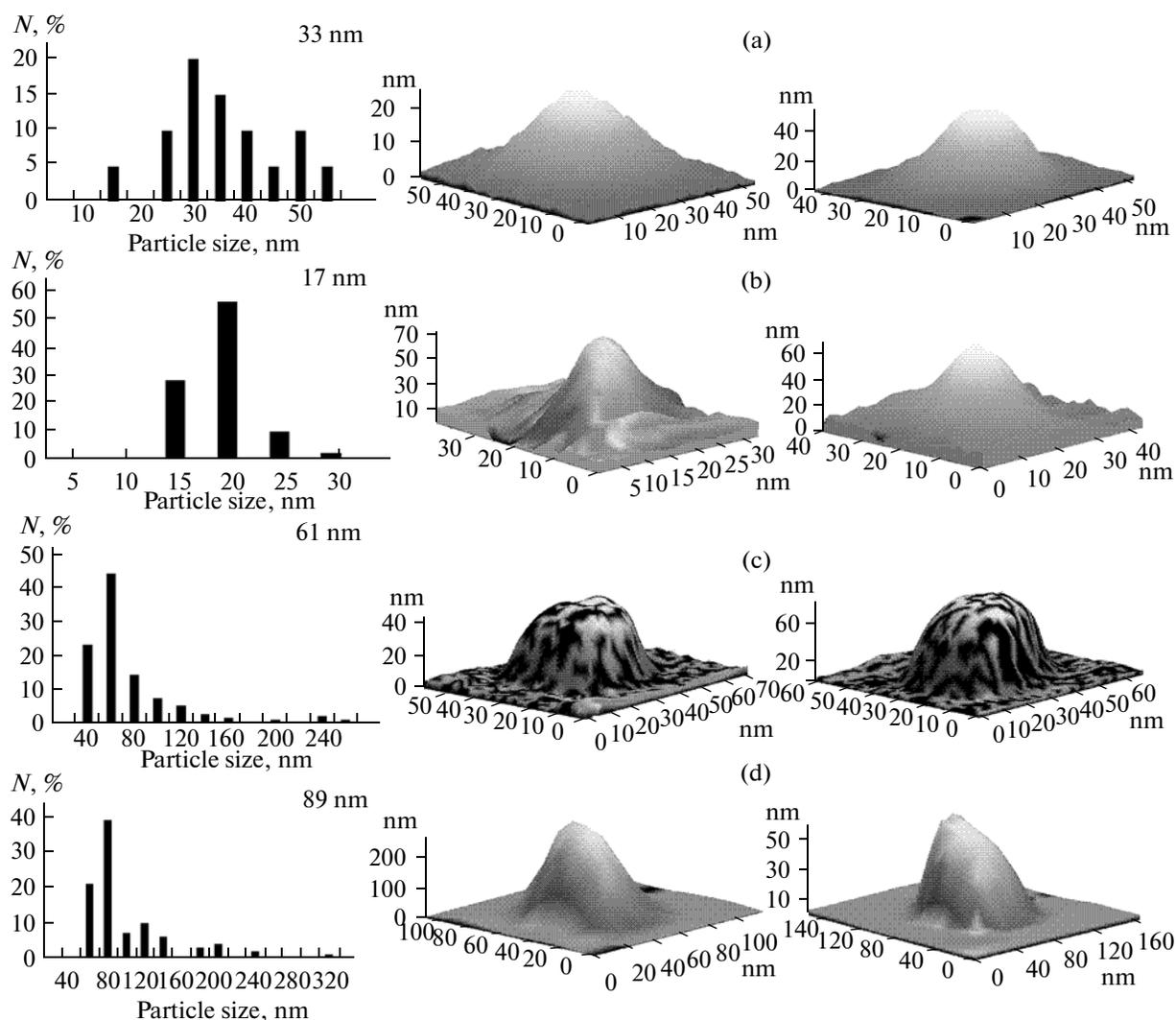
**Fig. 3.** Effect of synthesis conditions on the particle size distribution and three-dimensional images of amorphous silica nanoparticles.
