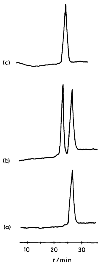
Figure 4. H.p.l.c. analysis of (a) yamogenin acetate (1), (b) a mixture of yamogenin and diosgenin, and (c) diosgenin. Conditions: column, TSKgel ODS-120T 250 \times 4 mm i.d.; solvent, 7% water in methanol, 1 ml/min; detector, UVILOG-5IIIA at 208 nm
