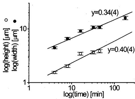
FIG. 2. Scallop growth with annealing time. Lateral width (from plane view images) and height (from cross section images) are evaluated separately.
