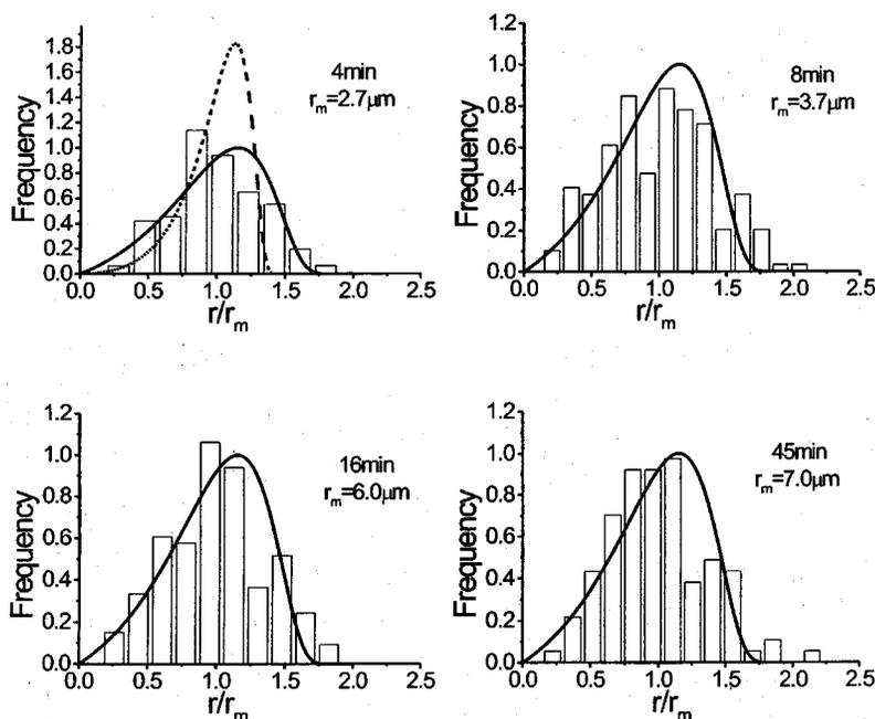
FIG. 3. Experimental size distributions (histograms) in comparison to Gusak's prediction (solid line). For the stage after 4 min reflow the classical LSW distribution is shown also (dashed line).
