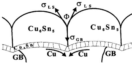
FIG. 5. Schematic of the solid/liquid interreaction zone.
