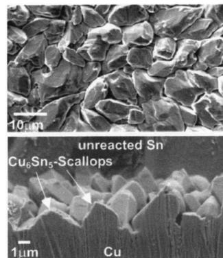
FIG. 1. Scanning electron microscopy: (top) plane view image of a Cu/Sn reaction zone after 8 min reflow., (bottom) cross-section image of a Cu/Sn reaction after 4 min reflow.
