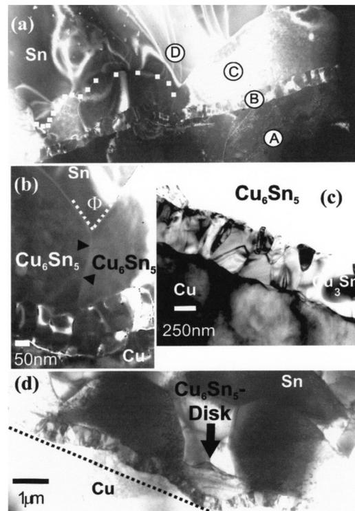
FIG. 4. TEM micrographs of a Cu/Sn specimen after 4 min reflow.
