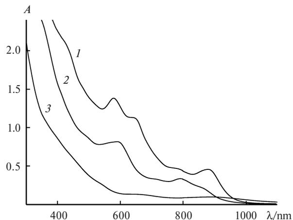
**Fig. 7.** The UV–Vis spectra of the trifluoromethyl EMF derivatives in toluene: Gd@C<sub>82</sub>(CF<sub>3</sub>)<sub>5</sub>, isomer 1 (*1*); Gd@C<sub>82</sub>(CF<sub>3</sub>)<sub>5</sub>, and isomer 2 (*2*); Gd<sub>2</sub>@C<sub>80</sub>(CF<sub>3</sub>) (*3*).
