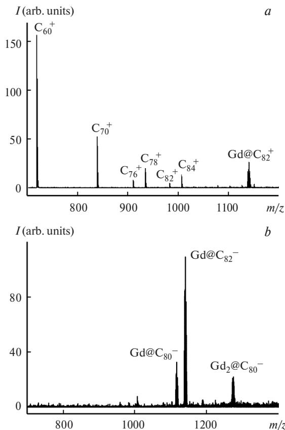
**Fig. 1.** The MALDI-TOF mass spectra of positive ions from the DCB extract of the soot (*a*) and negative ions from the DMF extract of the soot (*b*).
