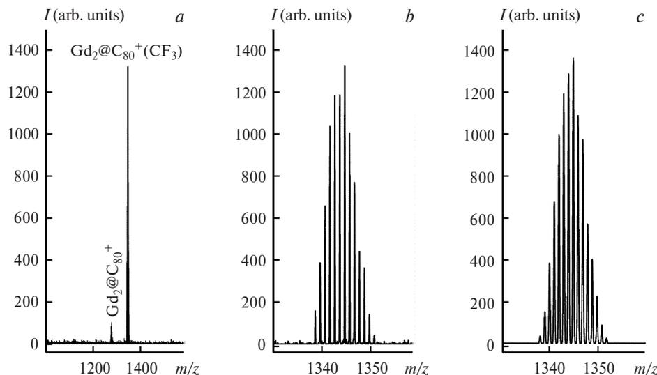
**Fig. 4.** The MALDI-TOF mass spectrum of positive ions of the pure trifluoromethyl derivative  $\text{Gd}_2\text{@C}_{80}(\text{CF}_3)$  (a), the observed isotope distribution of the peak with  $m/z$  1344 (b), and the theoretical isotope distribution for the  $\text{Gd}_2\text{@C}_{80}(\text{CF}_3)$  molecule (c).
