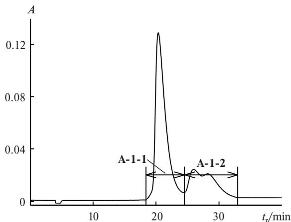
**Fig. 6.** The HPLC chromatogram of fraction **A-1** on the Regis Buckyclutcher column (toluene—hexane (40 : 60) mixture as eluent, eluting rate 12 mL min<sup>-1</sup>).
