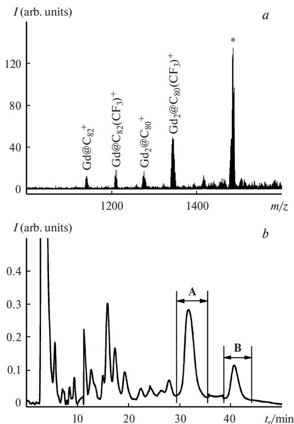
**Fig. 2.** The MALDI-TOF mass spectrum of positive ions (*a*) and the HPLC chromatogram (Cosmosil Buckyprep column, toluene as eluent, eluting rate  $18 \text{ mL min}^{-1}$ ) (*b*) of the trifluoromethylation products  $\text{Gd}@C_{82}(\text{CF}_3)_x$ . The peak marked by \* belongs to the  $\text{Gd}@C_{82}(\text{CF}_3)_5^+$  ions. Here and in Figs 3 and 6,  $t_r$  is the retention time.
