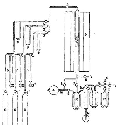
Figure 1. Butene Isomerization Apparatus
