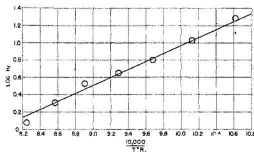
Figure 6. Relation between  $H_r$  and Temperature at Constant Apparent Gas Flow Rate of 480 Feet per Hour
