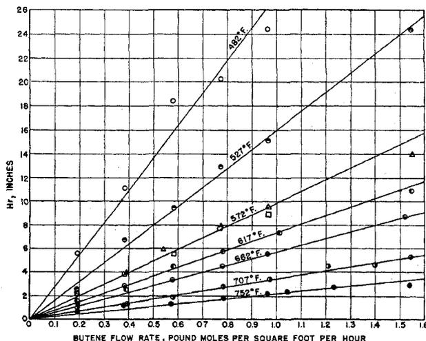
Figure 3. Relation between H<sub>r</sub> and Flow Rate at Various Temperatures
