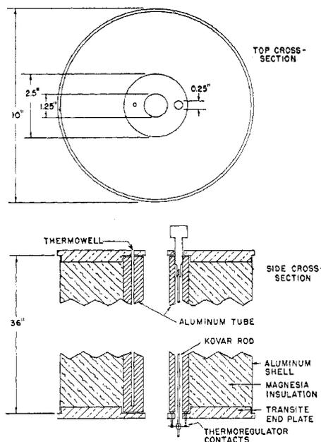
Figure 2. Details of Furnace Construction
