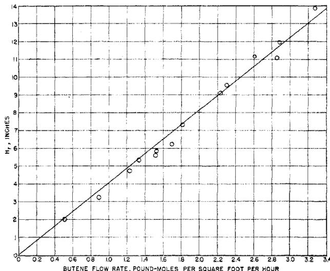
Figure 5. Effect of Higher Flow Rates on  $H_r$  at 350° C.
