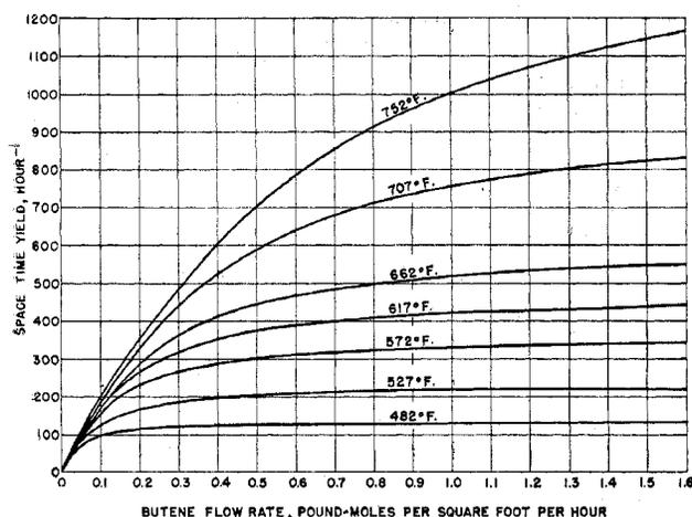
Figure 7. Variation of Space Time Yield with Flow Rate at Various Temperatures
