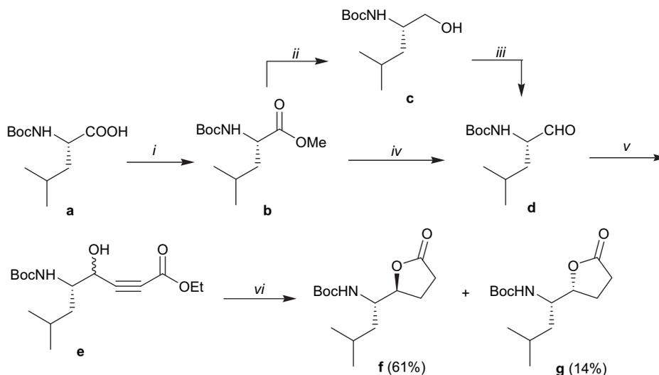
**Scheme 1.** Synthetic route to intermediate lactone **f**. Reagents and conditions: (i) NaHCO<sub>3</sub>, CH<sub>3</sub>I, DMF; (ii) NaBH<sub>4</sub>, CaCl<sub>2</sub>, THF/EtOH; (iii) Py·SO<sub>3</sub>, TEA, DCM/DMSO; (iv) DIBAL, toluene, 0 °C, 10 min; (v) ethyl propiolate, LDA (*n*-BuLi and *i*-Pr<sub>2</sub>NH, −23 °C in THF, 1 h), −78 °C, N<sub>2</sub>, 4.5 h; (vi) H<sub>2</sub>/Pd, 60 psi, EtOAc, then reflux in toluene/acetic acid (97.5:2.5 v/v).
