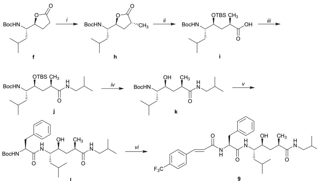
**Scheme 2.** Synthesis of compound **9** from lactone **f**. Reagents and conditions: (i) CH<sub>3</sub>I, LiHMDS, −78 °C; (ii) a. LiOH (1 N), THF; b. TBDMSCl, imidazole, DMF; (iii) isobutylamine, EDC, HOBt, DIPEA, DMF/CH<sub>2</sub>Cl<sub>2</sub>; (iv) *n*-Bu<sub>4</sub>N<sup>+</sup>F<sup>−</sup>, THF; (v) a. TFA/CH<sub>2</sub>Cl<sub>2</sub>; b. *N*-Boc-*L*-phenylalanine, EDC, HOBt, NMM, DMF; (vi) a. TFA/CH<sub>2</sub>Cl<sub>2</sub>; b. 4-(trifluoromethyl)cinnamic acid, EDC, HOBt, NMM, DMF.
