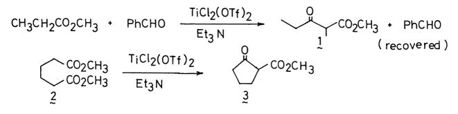
Several solvents were screened under the same condition employing  $Et_3N$  as a base (molar ratio of  $TiCl_2(OTf)_2$  : substrate :  $Et_3N = 1.1 : 1.0 : 1.1$ ), and 17% yield of product 3 was obtained along with 80% recovery of dimethyl adipate 2 in toluene. A trace amount of product 3 was given along with 61% and 75% recovery in ether and hexane respectively. The best result was obtained when dichloromethane was used, that is 45% yield of product 3 along with 55% recovery of 2.
