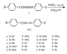
In this paper, using NaNO<sub>2</sub>-Ac<sub>2</sub>O as an oxidation system, ten acyl-diazenes have been synthesized from acylhydrazines in excellent yields (75.6-93.9%) under mild conditions. This method does not need a long time and is easy to operate. It is efficient and convenient. In the reaction we have found there is no inevitable relationship between the yields
