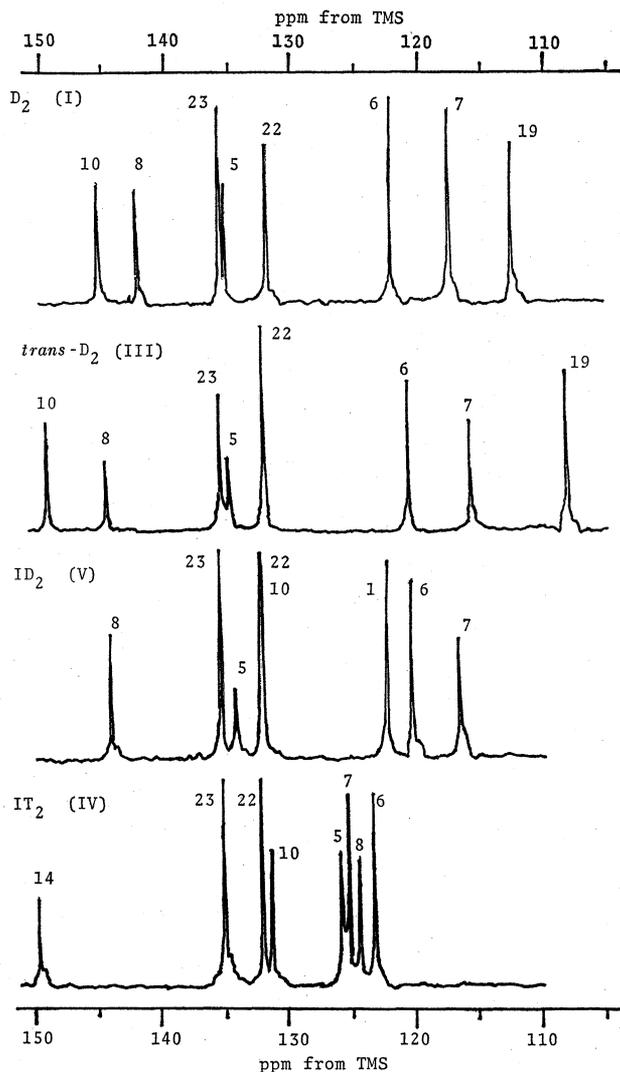
Fig. 2. Carbon-13 nmr spectra ( $sp^2$  region) of the four vitamin  $D_2$  isomers. [22.6 MHz, in  $CDCl_3$ ]
