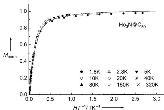
**Figure 2.** The experimental data  $M(H, T)$  for  $\text{Ho}_3\text{N@C}_{80}$  (symbols) corrected for the diamagnetic contribution and normalized to the saturation. The solid line represents the fitted Langevin function with a magnetic moment  $\mu = 21 \mu_B$ .
