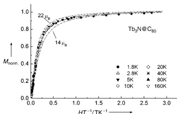
**Figure 3.** The experimental data  $M(H, T)$  for  $\text{Tb}_3\text{N}@C_{80}$  (symbols) corrected for the diamagnetic contribution and normalized to the saturation. The solid line represents the fitted Langevin function with a magnetic moment  $\mu = 17 \mu_B$ . The broken lines correspond to the normalized magnetization for  $\mu = 14 \mu_B$  and  $\mu = 22 \mu_B$ .
