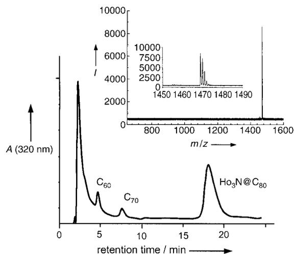
**Figure 1.** HPLC trace of the  $\text{Ho}_3\text{N@C}_{80}$  soot on a Buckyprep column with toluene as an eluent. The chromatogram shows the dependence of the optical absorption at  $\lambda = 320$  nm on the retention time, which reveals that  $\text{Ho}_3\text{N@C}_{80}$  is the main component of the soot. Inset: LD-TOF mass spectrum confirming the high purity of the  $\text{Ho}_3\text{N@C}_{80}$  sample.
