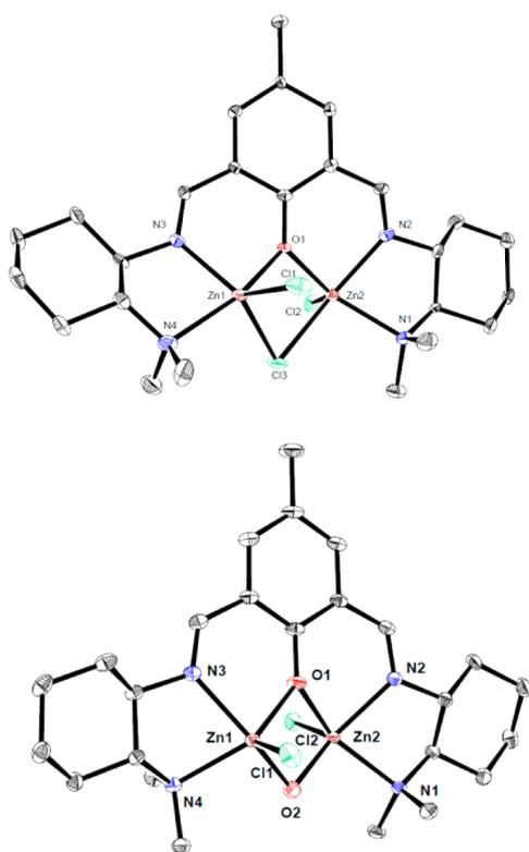
**Figure 2.** Solid-state structures of complexes (RR/RR)-4 (a, top) and (RR/RR)-5 (b, bottom) obtained by single-crystal X-ray diffraction. Thermal ellipsoids are set at 50% probability, and hydrogen atoms and solvent are removed for clarity. The unit cell for complex 4 contains two distinct diastereomers, 4a and 4b, differing in the positions of the chloride ligands around the zinc centers. Only 4a is depicted here.
