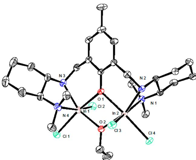
**Figure 1.** Solid-state structure of the complex (SS/SS)-1 [(SS/SS)-Δ,Δ] obtained by single-crystal X-ray diffraction. Thermal ellipsoids are set at 50% probability, and hydrogen atoms and solvent are removed for clarity.
