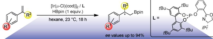
**Might of the phosphite:** The highly regio- and enantioselective hydroboration of challenging 1,1-disubstituted olefins is achieved by using iridium catalysts modified with chiral phosphite-based phosphinoxazoline ligands. Use of the biaryl phosphite moiety in the
